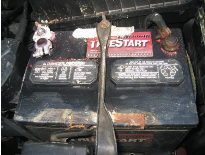
FIGURE 4.18 Corrosion due to electrochemical reaction.
