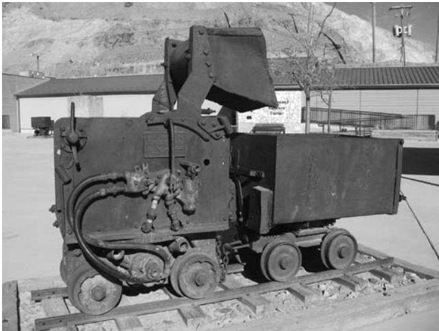
FIGURE 4.19 (See color insert following p. 142.) General corrosion observed on a mining cart.
