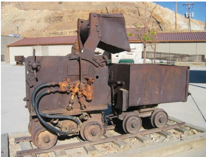
FIGURE 4.19 General corrosion observed on a mining cart.
