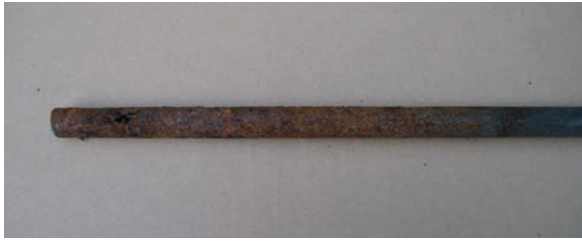
FIGURE 7.6 Uniform corrosion on a steel tube.
