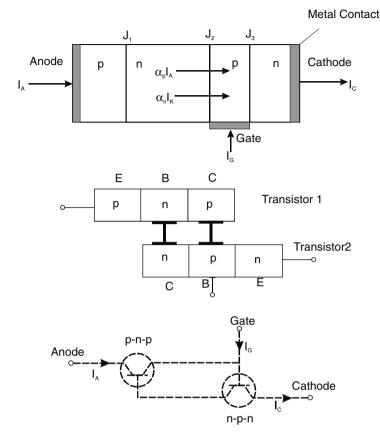
Fig. 4.22. Structure of thyristor, and two-transistor equivalent circuit
