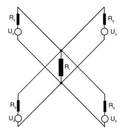
Fig. 7.1. Schematic representation of power addition by parallel switching of several generators to a common load ( $R_{\rm L} = R_{\rm g}/n$ ; n = number of units)
