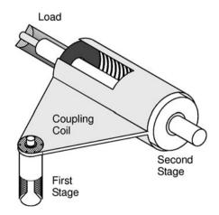
Fig. 10.19. Two-stage cascade system, inductively coupled
