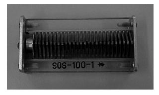
Fig. 4.50. 100 kV semiconductor-opening-switch (SOS) stack
