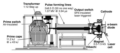
Fig. 11.6. One half of the ELECTRA pulsed-power system: 500 kV, 100 kA, 100 ns flat-top electron beam, 5 Hz repetition capability
