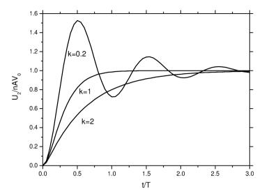
**Fig. 6.20.** Response of a pulse transformer to a voltage step for different degrees of damping  $\left(A = (R_2/n^2)/(R_g + R_2/n^2), n = N_2/N_1, k = \left[R_g/L_1 + 1/(R_2/n^2C)\right]T/4\pi, T = 2\pi \left(L_1(CA)^{1/2}\right)\right)$
