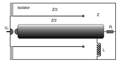
Fig. 7.6. Schematic representation of a classical Blumlein line
