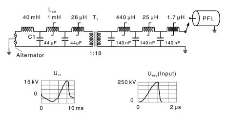
Fig. 8.7. Equivalent-circuit model of the RHEPP pulse generator
