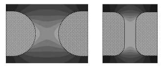
Fig. 2.9. Distribution of equifield surfaces between two different electrode configurations. The greyscale steps represent 10% changes in the field strength
