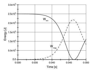
Fig. 3.22. Evolution of the kinetic energy  $W_{\text{kin}}$  and the magnetic energy  $W_{\text{mag}}$  for a self-exciting homopolar generator
