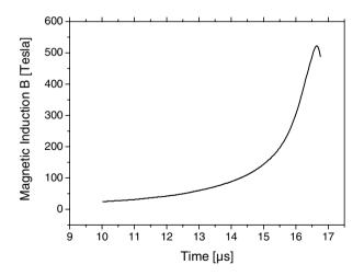
Fig. 10.16. Representative waveform from a cylindrical implosion experiment of the kind shown in Fig. 10.15
