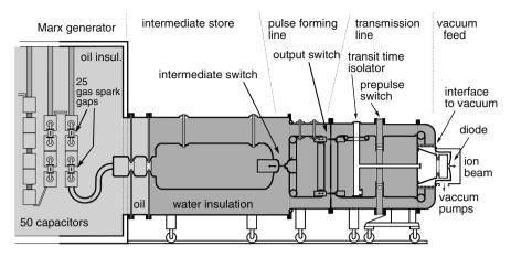
Fig. 8.1. Schematic illustration of the 1.5 TW pulse generator KALIF. The data for the pulse at the vacuum interface are: power = 1.5 TW, voltage = 1.7 MV, pulse duration = 50 ns, pulse energy = 75 kJ, electrical efficiency = 30%
