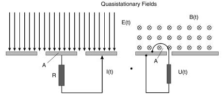
Fig. 9.1. Basic types of sensors: electric and magnetic dipoles
