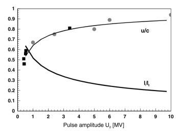
Fig. 6.15. Wave front propagation velosity and loss current in a self-magnetically insulated vacuum line as a function of pulse amplitude (*squares*, experimental results [Baranchikov et al. 1978]; *circles*, results from PIC-code simulations [Poukey and Bergeron 1978])
