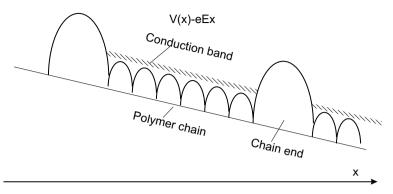
Fig. 2.23. Band structure for a section of an extended polymer chain coinciding with the field direction. At very large fields, excess electrons liberated from traps can move quasi-freely in a conduction band along the chain. At the chain ends, they must tunnel through a potential well to reach the next chain
