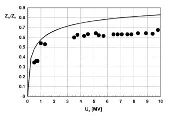
Fig. 6.13. Relative impedance  $Z_{in}/Z_0$  of a vacuum line as a function of pulse amplitude
