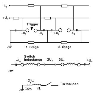
Fig. 3.10. Marx generator with bipolar charging. Compared with the simple circuit of Fig. 3.9, only half the number of switches are required. Stray capacitances have been neglected again
