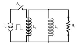
Fig. 4.40. Superconducting energy storage device  $L_{\rm s}$  with a superconducting opening switch activated by a pulsed-magnetic field coil  $L_{\rm a}$ , which creates a field above the critical value in a section of the superconducting circuit. The resistance of this section must become larger than the load resistance  $R_{\rm L}$  to divert the current into the load effectively
