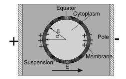
Fig. 10.1. Spherical cell in an external electrical field E
