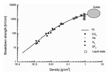
Fig. 2.1. Static insulation strength of various gases and liquids versus density [Cooke 1998]
