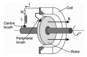
Fig. 3.20. Basic set-up of a self-exciting homopolar generator
