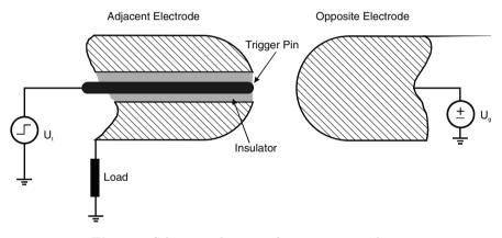
Fig. 4.8. Schematic drawing of a trigatron spark gap
