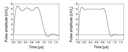
**Fig. 5.16.** Pulse voltage of a three-element (left) and five-element (right) Guillemin network into a matched load
