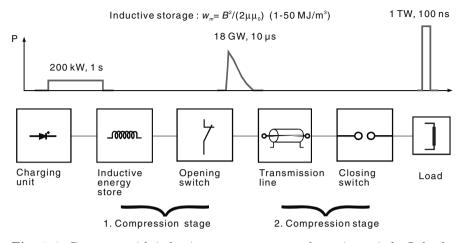
Fig. 1.4. Generator with inductive energy storage and opening switch. Only the first compression stage uses inductive storage. The later stages are capacitive and need a closing switch. As previously, we have assumed losses of about 50%
