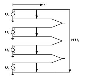
Fig. 7.2. Adding of voltage pulses by transit-time isolation
