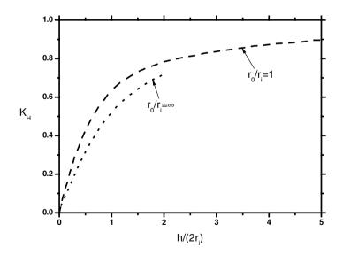
Fig. 10.13. Field factor  $K_{\rm H}$  as a function of  $h/2r_{\rm i}$  for  $r_{\rm o}/r_{\rm i} = 1$  [Bardotti et al. 1964] and  $r_{\rm o}/r_{\rm i} = \infty$
