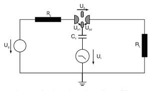
**Fig. 4.4.** Wiring diagram of a three-electrode spark gap ( $U_{\rm g}$  = generator voltage,  $U_{\rm t}$  = trigger voltage,  $U_{\rm b}$  = breakdown voltage,  $U_{\rm b1}$ ,  $U_{\rm b2}$  = breakdown voltages of the partial gaps,  $R_{\rm g}$  = generator impedance,  $R_{\rm L}$  = load impedance,  $C_{\rm c}$  = coupling capacitor)
