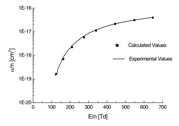
**Fig. 2.2.** Comparison of experimental data for  $\alpha/n$  in nitrogen with values calculated from basic cross-section data [Meek and Craggs 1978]. Here, the old unit Townsend (Td) has been used, where  $1 \text{ Td} = 10^{-17} \text{ V cm}^2$
