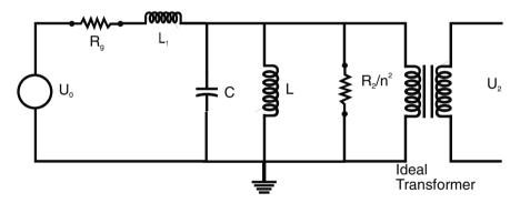
Fig. 6.19. Equivalent-circuit model of a real transformer
