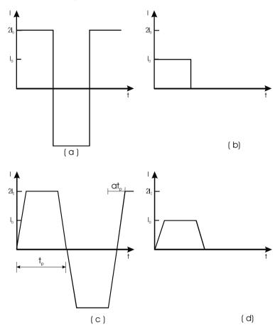
Fig. 5.13. Design concept for a Guillemin network. (a) Output current of an ideal transmission line into a short circuit. (b) Output current of the same line into a matched load. (c) Trapezoidal pulse from a Guillemin network with a short-circuit load. (d) Ideal discharge of a Guillemin network into a matched load
