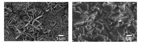
**Fig. 11.4.** Surface morphology of the oxide scale grown on the surface of a NiCrAlY oxidation protection layer after 200 h at 950°C. *Left*, with conventional polishing of the plasma-sprayed layer; *right*, with GESA electron beam treatment
