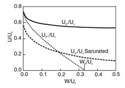
Fig. 11.13. Critical voltages  $U_{2^*}$  and  $U_{2^{**}}$  in the post-acceleration gap as a function of the injected ion energy W, normalized to the critical voltage  $U_c$  for magnetic insulation (from [Slutz and Desjarlais 1990])
