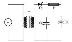
Fig. 6.21. Schematic of a resistive charging unit (D = rectifying diode,  $C_s =$  smoothing capacitor)
