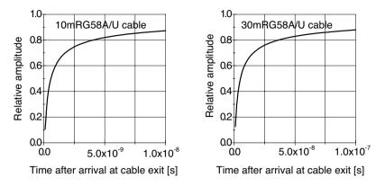
Fig. 5.6. Relative amplitude of a step pulse at the exit of a 10 and a 30 m long RG 58A/U coaxial cable. ( $Z_0 = 50 \Omega$ ,  $k = 1.14 \times 10^{-6}$  (at 1 GHz),  $c/c_0 = 0.659$ )
