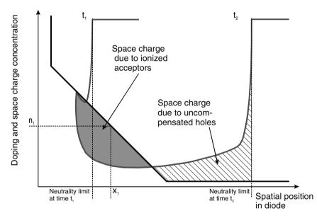
Fig. 4.49. Schematic illstration of the movement of the plasma front and the formation of space charge in a semiconductor opening switch during reverse-current operation
