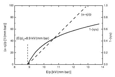
Fig. 2.4. Effective ionisation coefficient  $(\alpha - \eta)/p$  and weight function  $1 - (\eta/\alpha)$  describing the probability that an electron creates further avalanche electrons, for SF<sub>6</sub>
