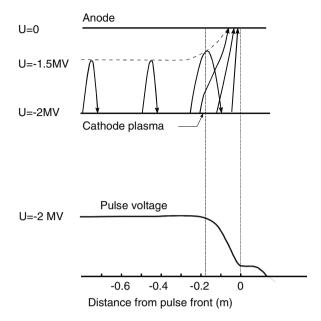
Fig. 6.6. Electron trajectories and corresponding development of the pulse voltage during propagation in a transmission line with progressing self-magnetic insulation
