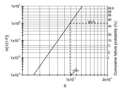
**Fig. 2.25.** Weibull distribution plot of (2.58). On the *right axis*, the cumulative failure probability F corresponding to each value of  $\ln[1/(1-F)]$  is plotted. For F = 63%, one can read  $\langle S \rangle$  from the abscissa. The gradient of the double logarithmic plot gives the exponent B
