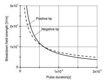
Fig. 2.19. Mean pulsed breakdown strength in water for a point-plane or edgeplane geometry. These graphs have been derived from the empirical formulae given in (2.48), which were derived for pulse durations greater 100 ns and pulse amplitudes between 0.1 and 1 MV. The plot has been calculated for a gap of 4 cm
