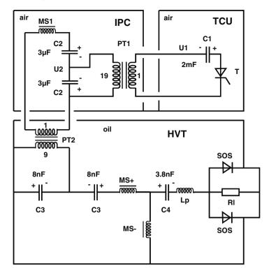
Fig. 8.8. A 1 MV generator with repetition rate capability based on semiconductor opening switches, consisting of a thyristor-controlled charging unit (TCU), an intermediate transformation and compression stage (IPC), and a high-voltage transformation and compression stage (HVT)
