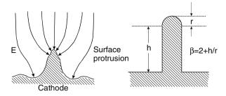
Fig. 6.4. Field distribution at the tip of a whisker, and a simple model to calculate the field enhancement factor  $\beta$
