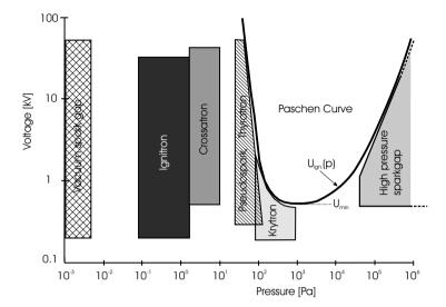
**Fig. 4.1.** Range of gas pressures and operating voltages for various types of gas switches. In addition, the Paschen curve for air is shown for a fixed gap width of 3 mm. Above this curve, switch operation becomes impossible since the breakdown strength is exceeded
