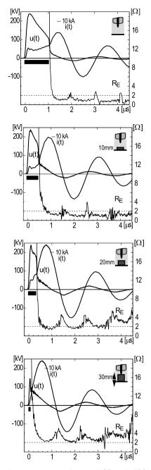
Fig. 12.9. Voltage and current wave shapes U(t) and I(t) and the derived spark channel resistance  $R_s$  for various conditions in the interelectrode gap. For this series of measurements, an interelectrode distance of 30 mm was chosen. The voltage traces shown have not been corrected for the inductive voltage drop
