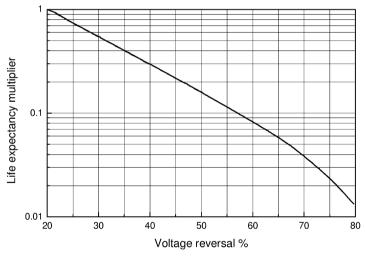
Fig. 3.7. Voltage reversal coefficient of life
