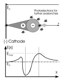
**Fig. 2.6.** Effect of space charge produced by an avalanche on the electric field in a gap. Ions are rather immobile and form a dipole field together with the electrons removed from the ions. This field will enhance the initially applied electric field  $E_0$  at the avalanche head
