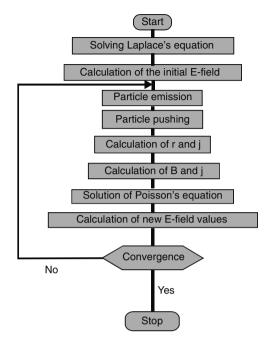
Fig. 6.7. Flow diagram of a particle-in-cell (PIC) code
