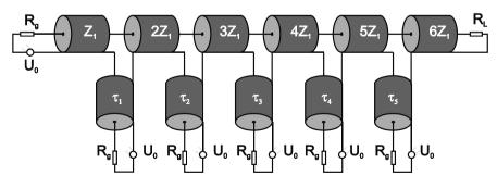
Fig. 7.5. Model for simulation of the voltage adder of Fig. 6.3 with the circuit program LEITER  $\,$
