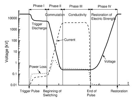
Fig. 4.2. Evolution of voltage, current, and power loss in a gas-filled switching system
