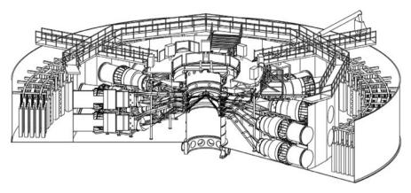
**Fig. 8.4.** Schematic illustration of the Z-Machine for driving Z-pinches, located at Sandia National Laboratory
