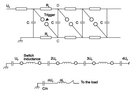
Fig. 3.9. Marx generator circuit with unipolar charging through the resistors  $R_{\rm L}$  (*top*). Configuration of Marx after firing of all switches (*middle*). Lumped circuit model of erected Marx generator (*bottom*)
