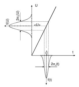
Fig. 4.14. Relation between the standard deviation of voltage breakdown  $\sigma_{\rm a}(U)$ and the time variance  $\sigma_{\rm a}(t)$
