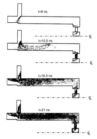
Fig. 6.8. Evolution of electron flow in a self-magnetically insulated transmission line terminated with an electron diode
