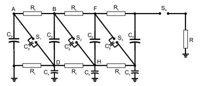
Fig. 3.11. Marx generator with stray capacitances  $C_{\rm s}$  between stage capacitors and ground, and  $C_{\rm g}$  across switches. Stray capacitances between A, B, F, etc. and ground have been assumed to be negligible
