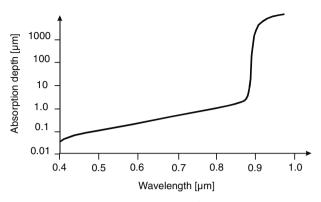
Fig. 4.32. Optical absorption depth in GaAs as a function of wavelength
