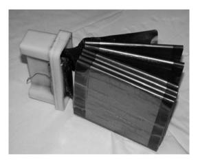
Fig. 3.5. 60 kV,  $0.2 \mu$ F power capacitor consisting of six roll-ups. The case has been dismantled. The capacitor terminals are embedded in the plastic head on the left
