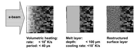
Fig. 11.1. Schematic illustration of e-beam surface modification. Owing to the high cooling rate caused by heat conduction into the cold bulk material, structural and phase changes can occur, changing the hardness, the wear resistance, and the corrosion and oxidation resistance
