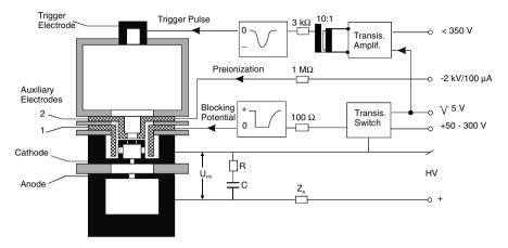
Fig. 4.17. Pseudospark switch arrangement, including a schematic of the trigger section. Triggering is achieved with the help of a glow discharge created in the upper part of the switch. (All metallic parts are either shown in black or cross-hatched. Insulators are grey.) [Frank and Rath 1990]
