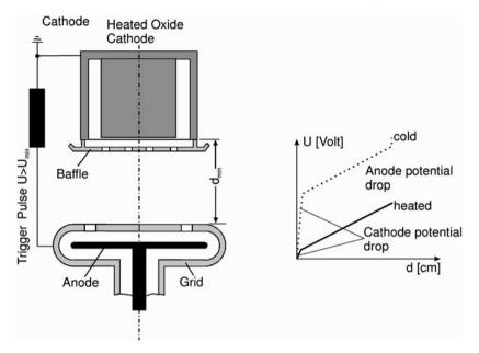
Fig. 4.15. Principal features of a thyratron with heated cathode (*left*), and potential drop with a heated cathode (*solid line*) and without one (*right*). The grid surrounds the anode such that the pd value excludes the possibility of a long-distance discharge
