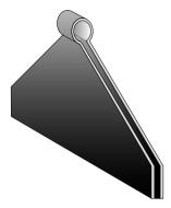
Fig. 10.12. Single-turn coil with converging low-impedance stripline
