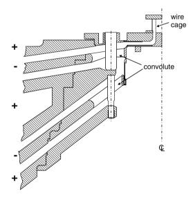
Fig. 8.5. Post-hole convolute in the Z-Machine
