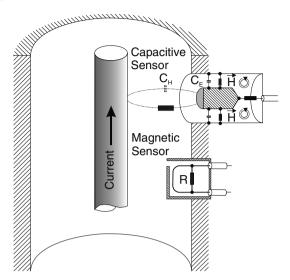
Fig. 9.3. Scheme of capacitive and magnetic sensors integrated into a coaxial line
