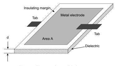
Fig. 3.1. Elements of a parallel-plate capacitor
