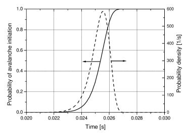
Fig. 2.10. Probability of avalanche initiation and the corresponding probability density in a 1 cm gap insulated with dry nitrogen. The voltage across the homogeneous gap rises at a rate of  $6 \,\mathrm{MV/s}$
