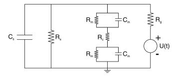
**Fig. 10.2.** Equivalent circuit of a biological cell.  $R_{\rm m}$  = membrane resistance,  $C_{\rm m}$  = membrane capacitance,  $R_{\rm s}$  = resistance of suspension,  $C_{\rm s}$  = stray capacitance bypassing the cell,  $R_{\rm g}$  = generator impedance, U(t) = time-dependent voltage pulse
