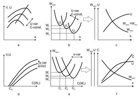
Fig. 12.14. Schematic representation of a procedure to determine the optimum voltage amplitude and generator capacitance as a function of interelectrode distance s for the minimum energy consumption  $W_{\text{spec}}$  (after [Sjomkin et al. 1995])
