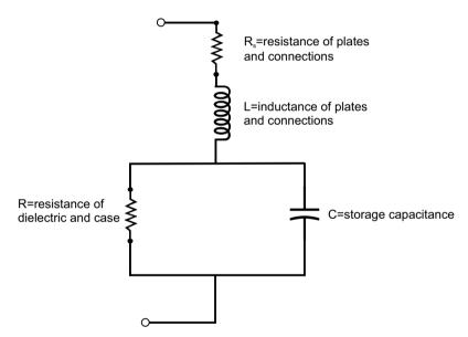
Fig. 3.2. Lumped circuit model of a capacitor
