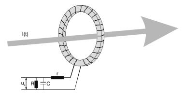
Fig. 9.5. Schematic representation of a Rogowski coil
