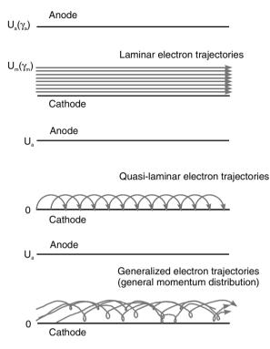
Fig. 6.10. Conceivable electron trajectories in a parallel plate vacuum transmission line
