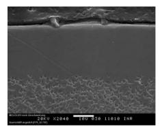
Fig. 11.3. MCrAlY oxidation protection layer after pulsed-electron-beam treatment. The *upper part* of the electron micrograph shows the restructured surface layer. *Lower part*: original MCrAlY two-phase structure
