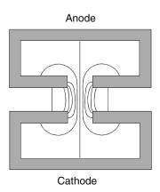
Fig. 4.16. Electric-field configuration in a two-electrode pseudospark system
