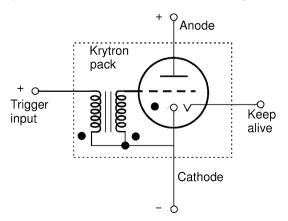
Fig. 4.20. Schematic of krytron pack including a trigger transformer
