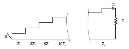
Fig. 7.8. Cumulative pulse line with stepwise-increasing impedance
