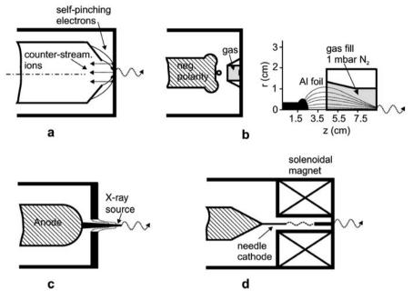
Fig. 11.9. Diode sources for the production of intense pulsed X-ray radiation. (a) Pinched-beam source; (b) paraxial diode: electron trajectories self-pinching in the gas cell are shown to the right of the geometric scheme; (c) rod pinch diode; (d) magnetically immersed diode
