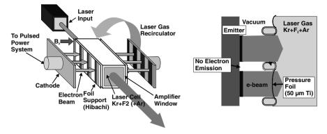
Fig. 11.7. Principal features of an electron-beam-pumped KrF laser
