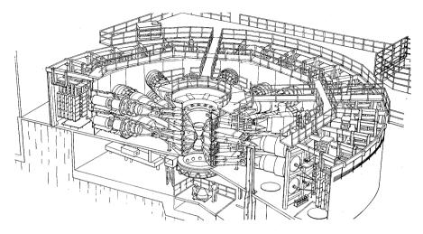
Fig. 8.2. Perspective drawing of the multimodular generator PBFA 2
