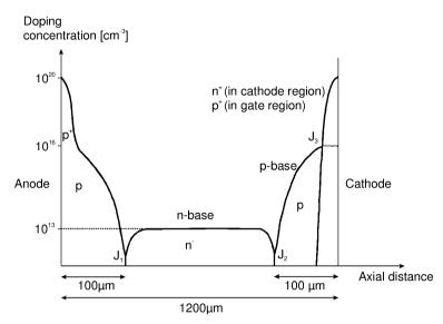
Fig. 4.23. Doping profile of the layers of a thyristor
