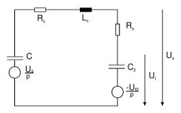
Fig. 4.11. Equivalent circuit of the discharge configuration after breakdown of the first switch gap
