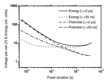
Fig. 10.4. Pulse voltage and energy for irreversible breakdown as a function of the minimum pulse width for two different internal time constants  $R_{\rm c}C_{\rm m}$
