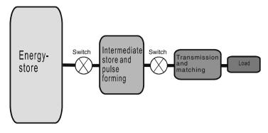
Fig. 1.2. General scheme of a pulsed-power generator
