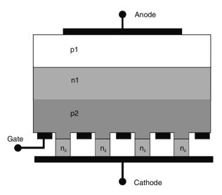
Fig. 4.27. Structure of a GTO thyristor
