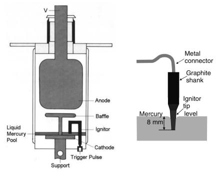
Fig. 4.19. High-voltage ignitron with splash baffle, and with a schematic illustration of the ignitor pin set-up. An enlarged view of the mercury contact to the trigger pin is shown on the right
