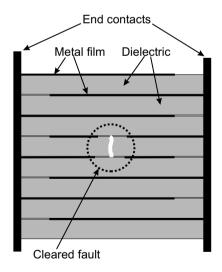
Fig. 3.8. Metallized-film capacitor stack with cleared breakdown spot
