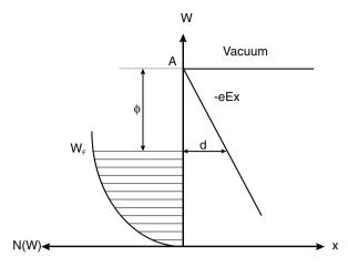
Fig. 6.3. Illustration of high-field electron emission by tunnelling. The vertical axis represents also the boundary between metal and vacuum
