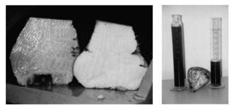
Fig. 10.6. Left photograph: Sugar beets before (right) and after (left) treatment with pulsed electric fields. Right photograph: corresponding yields of juice obtained by cold pressing at 32 bar
