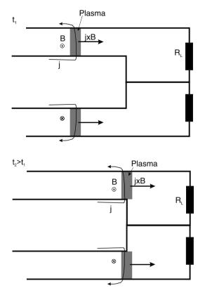
**Fig. 4.44.** General scheme of a plasma flow switch: conduction phase (*top*) and beginning of opening phase (*bottom*)
