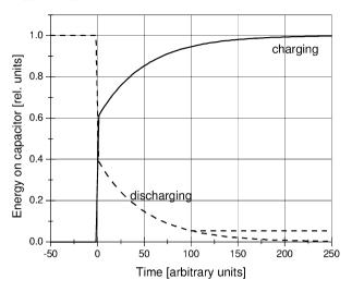
**Fig. 3.4.** Typical response of a dielectric to a square-wave voltage pulse (*curve labelled 'charging'*) and to sudden switching of an ideal capacitor into an ideal short circuit (*curve labelled 'discharging'*)
