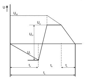
Fig. 4.7. Breakdown sequence in the longitudinal-plasma-triggering mechanism
