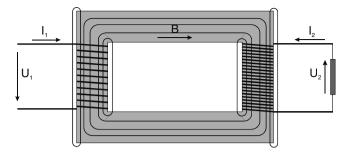
Fig. 6.17. Voltages, currents, fields, and flux in a transformer
