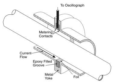
Fig. 9.8. Cross-section of a CVR integrated into the outer conductor of a coaxial transmission line
