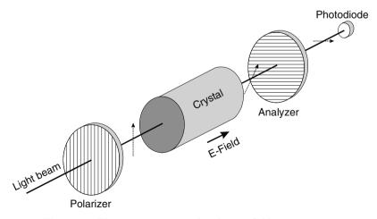
Fig. 9.10. Electro-optic sensor for electric-field measurement
