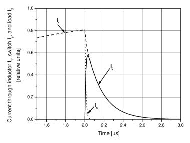
**Fig. 3.19.** Inductor, load, and switch currents in a generator based on inductive storage and opening switches.  $(L_1 = 1 \,\mu\text{H}, L_2 = 0.1 \,\mu\text{H}, R_g = 1 \,\Omega, R = 0.1 \,\Omega, R_s = 10 \,\Omega, R_l = 5 \,\Omega)$
