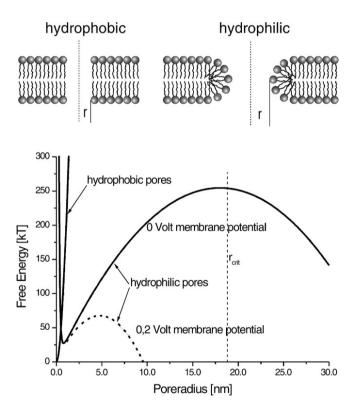
**Fig. 10.3.** Free energy F of pore formation as a function of pore radius for hydrophobic and hydrophilic pores. For hydrophilic pores, F is shown for two membrane potentials (0 and 0.2 V). During the pulse, the pore radius must grow above  $r_{\rm crit}$  if a permanent irreversible opening is to be obtained. Otherwise, the pore is reversible, i.e., the cell can heal it after disappearance of the membrane potential
