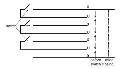
Fig. 7.7. Schematic representation of a generalised Blumlein line
