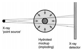
Fig. 11.8. Schematic illustration of point-projection radiography of fast-moving objects
