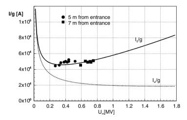
Fig. 6.11. Reduced wall current  $I_{\rm w}$  and total current  $I_0$  in a magnetically insulated vacuum line as a function of the sheath potential  $U_{\rm m}$  for  $U_0 = 1.8$  MV. The symbols represent experimental data obtained in a 7.5 m long parallel-plate line [Wang and DiCapua 1980]
