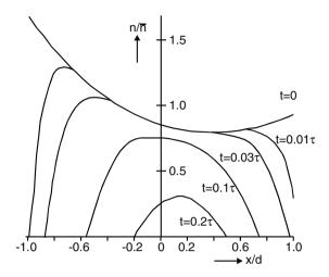
Fig. 4.46. Sweeping out of carriers from the swamped zone by a strong reverse current  $j_{\rm R} = 10 j_{\rm F} \ (\mu_{\rm n} = 3\mu_{\rm p}, \ d = L_{\rm d})$
