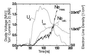
Fig. 11.11. Diode voltage  $U_d$ , ion current  $I_{ion}$ , and electron density Ne at a position 3 mm from the anode surface. Also shown is the electron density  $Ne_{calc}$  derived from  $U_d$  and  $I_{ion}$  using an analytic model for the saturated (constant-density) electron distribution
