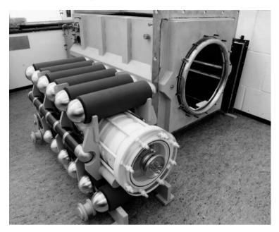
Fig. 12.8. Photograph of a 400 kV, 1.8 kJ Marx generator designed to operate at 10 Hz with a component lifetime of  $10^8$  pulses. The generator discharge period is  $2.5\,\mu s$
