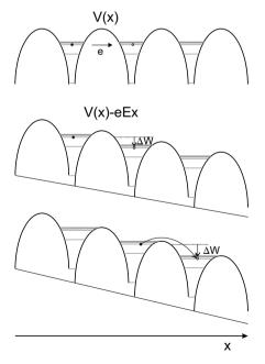
Fig. 2.15. Transfer of excess electrons between molecular states by resonance tunnelling under the influence of an electric field
