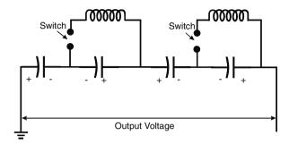
Fig. 3.14. Simplified representation of an LC Marx generator
