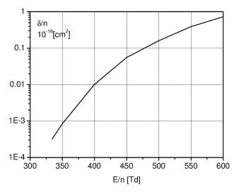
Fig. 2.8. Detachment coefficient d/n for SF<sub>6</sub> ions in SF<sub>6</sub> [Hilmert and Schmidt 1991]
