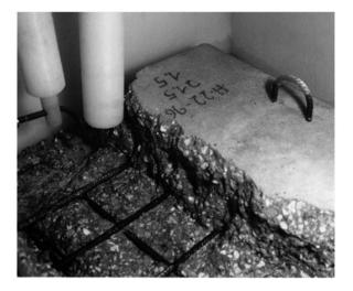
Fig. 12.15. View of a block of reinforced concrete with the surface layer removed. Here the two-electrode system shown in the upper left corner of the photograph was used
