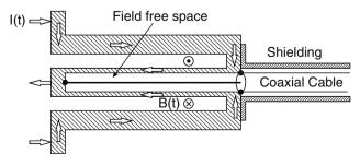
Fig. 9.7. Cylindrically symmetric shunt providing a field-free space at the position of the metering contacts
