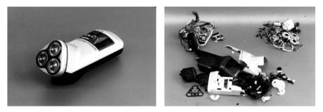
Fig. 12.16. Pulsed electric discharges can be used to separate metallic and dielectric components of electrical appliances. The right photograph shows the result of treatment of an electric razor with a few pulses
