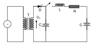
Fig. 6.22. One-cycle resonant charging system
