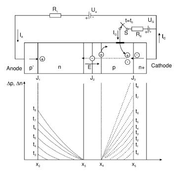
Fig. 4.24. Time sequence of charge carrier densities during switch-on [Gerlach 1979]
