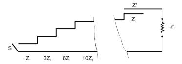
Fig. 7.9. Cumulative transmission line combined with Blumlein configuration
