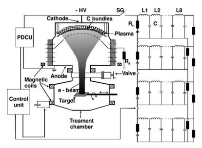
Fig. 11.2. Schematic illustration of the pulsed-electron-beam facility GESA (electron energy 50–150 keV, electron current  $\leq 700$  A, energy flux on target  $\leq 50 \text{ J/cm}^2$ ). 'PDCU' stands for 'pulse duration control unit', which serves to control the pulse duration
