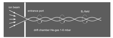
Fig. 11.14. Schematic illustration of self-pinched ion beam transport
