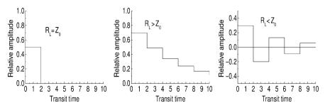
Fig. 5.9. Pulse shapes obtained for three different terminations of a cable
