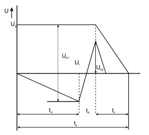
Fig. 4.5. Evolution of the voltages at the trigger and main electrodes of a threeelectrode spark gap using longitudinal overvoltage triggering ( $t_a$  = trigger actuating time,  $t_d$  = switching delay,  $t_c$  = commutation time,  $t_s$  = switching time)
