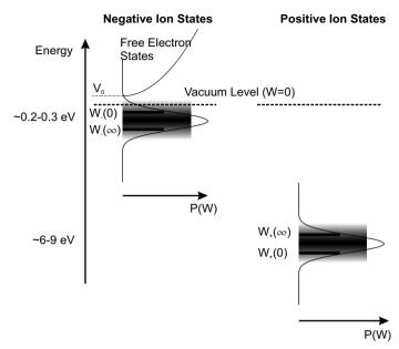
**Fig. 2.14.** Electronic energy states for positive and negative ions in a liquid.  $W_{-}(\infty)$  and  $W_{+}(\infty)$  correspond to fully localised states due to complete collective polarisation. The energy levels are broadened into Gaussian distributions P(W) by thermal agitation. Electrons with energies greater than  $V_0$  can be considered as quasi-free
