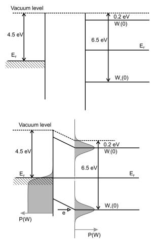
Fig. 2.17. Conditions at an interface between a metal cathode and a dielectric liquid, before (top) and after (bottom) contact. Electron transfer to negative-ion states  $W_{-}$  is energetically difficult, but easy to positive-ion states  $W_{+}$ . However, the transfer rate depends on the number of empty states in the liquid boundary layer. An overlap between occupied free-electron states in the metal and empty  $W_{-}$  states in the liquid boundary may occur at high electric fields
