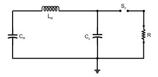
Fig. 3.13. Peaking-capacitor circuit
