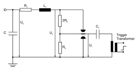
Fig. 4.9. Circuit diagram of three-electrode trigger set-up
