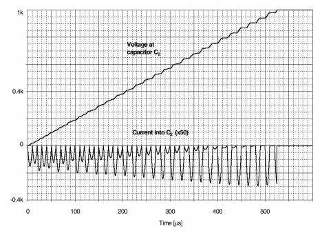
Fig. 6.24. Resonance-current pulses delivered to the load capacitor in Fig. 6.23 (*bottom* part), and voltage build-up (parameters:  $U_{\rm DC} = 100$  V, inverter frequency = 25 kHz, transformer step-up = 10)
