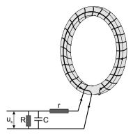
Fig. 9.6. Compensated Rogowski coil to eliminate the portion of the signal created by the flux penetrating the main opening of the coil
