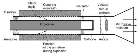
Fig. 10.18. Exploding flux compression generator driving a vircator for the production of intense pulsed microwave radiation
