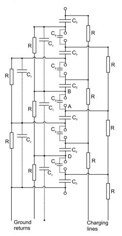
Fig. 3.12. n = 2 Marx generator with capacitive coupling across every two gaps
