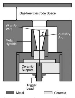
Fig. 4.21. Sectional view of a triggered vacuum switch with a coaxial plasma gun for triggering
