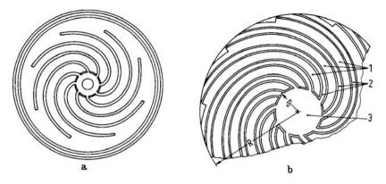
Fig. 4.28. Spiral gate stripe geometry of a high-current thyristor [Gerlach 1979]. 1, emitter stripes; 2, gate leads, 3, central gate contact
