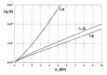
Fig. 6.12. Reduced minimum current  $I_{\min}/g$ , critical current  $I_{cr}/g$ , and saturation current  $I_p/g$  in a self-magnetically insulated vacuum line as a function of the anode potential  $U_0$
