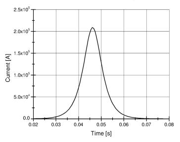
Fig. 3.21. Output current pulse of a homopolar generator
