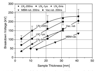
Fig. 12.17. Dependence of the breakdown voltage of  $LN_2$  on sample thickness for various ramp rates. Also shown is the breakdown voltage of rubber at cryogenic temperatures (from [Kurets et al. 1995])
