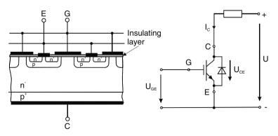
Fig. 4.30. General structure of an IGBT, and an IGBT switch set-up with an anti-parallel diode
