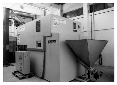
Fig. 12.12. FRANKA-1 before shipment to an incineration plant. FRANKA-1 is used to separate metallic components from the ash and to immobilise heavy metals in the ash
