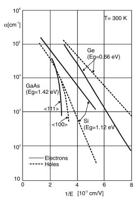
Fig. 4.31. Ionisation rate coefficients  $\alpha_n$  and  $\alpha_p$
