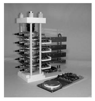
Fig. 4.29. Four-stage repetitive thyristor switch with integrated free-running diode and trigger circuit. Maximum operating voltage, 10 kV; peak current, 30 kA; maximum current rise,  $20 \text{ kA}/\mu s$ ; repetition rate, 10-50 Hz. Water-cooling bodies are visible between the thyristor units. A single unit with a trigger circuit but without water cooling is shown at the *bottom*
