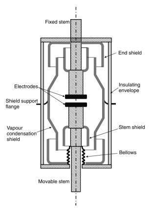
Fig. 4.38. Cross-section of a typical vacuum interrupter [Lafferty 1980]
