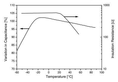
Fig. 3.3. Variation of capacitance and insulation resistance versus temperature for a capacitor using oil-impregnated paper as the dielectric
