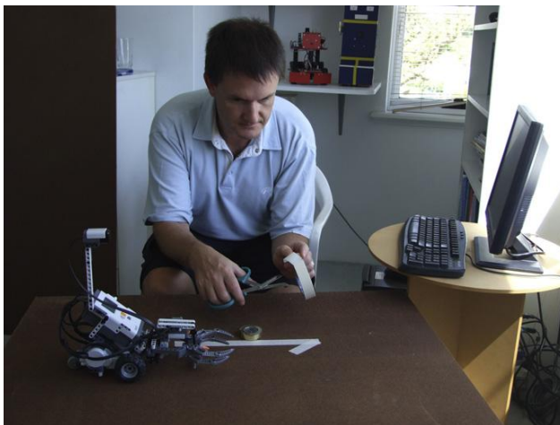
FIGURE 54.3 Getting ready to test a magnetic sensor. The direction of magnetic north is being marked on the base board, using masking tape and taking bearings from a small pocket magnetic compass. The sensor is mounted on a mast to keep it clear of the magnetic fields of the motors. This robot has a pair of jaws for picking up and carrying objects. The jaws are opened and closed by the robot’s third electric motor.
