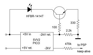
Figure 6. The keep-alive current sense circuit
