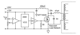
Figure 7. The Class-E power converter
