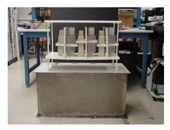
Figure 4. The Marx bank and its components
