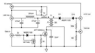
Figure 5. The Flyback trigger circuit
