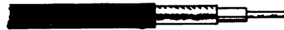
coaxial cable (From left to right: insulating jacket, woven outer conductor, low-loss insulating sleeve, inner conductor.)
