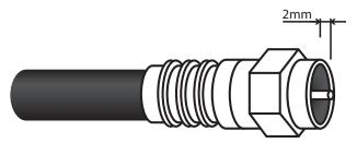
7. Slide on Connector, leaving 2mm of centre conductor protruding. Dielectric should also be flush with the bottom of the nut.
