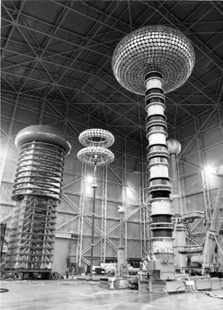
Figure 2.19 2.2 MV series resonant circuit (Hitachi Research Laboratory, supplied by Hipotronix, Brewster, USA)
