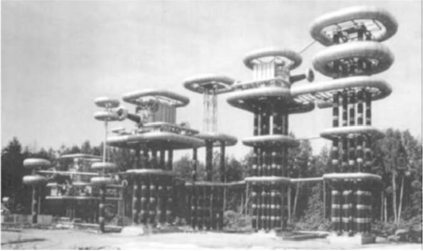
Figure 2.16 (b) Cascaded testing transformers with metal tanks and coolers. Total voltage 3000 kV, 4 A (courtesy HIGH-VOLT Dresden, Germany)
