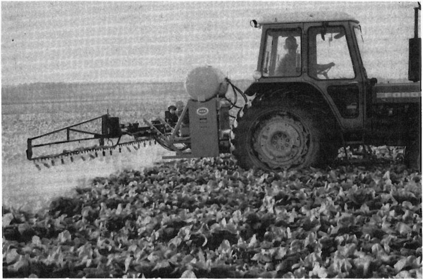
Figure 14 Tractor-mounted electrostatic crop sprayer incorporating thirty embedded electrode air assisted induction nozzles for row-crop pest control. (Photograph courtesy of Electrostatic Spraying Systems, Inc.)
