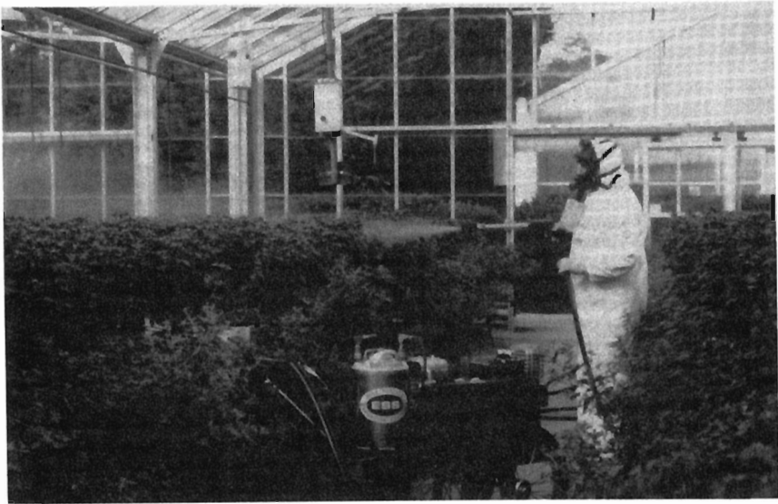
Figure 13 Hand-directed electrostatic sprayer for greenhouse pest control. (Photograph courtesy of Electrostatic Spraying Systems, Inc.)
