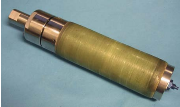
Fig. 14.1 Photograph of a prototype piezoelectric High Voltage Generator (HVG) developed by Diehl BGT Defence GmbH and Company in Germany.
