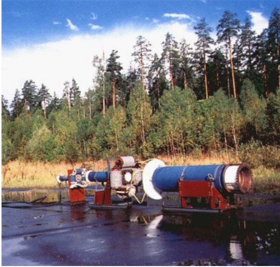
Fig. 6.14 Series connected FCG cascade at the All Russian Institute of Experimental Physics. The FCGs are connected via open-air transformers.
