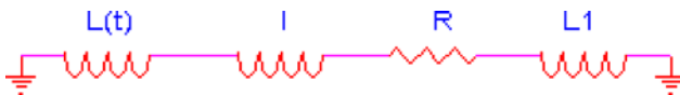
Fig. 5.3 Circuit diagram for an FCG (variable inductor) powering a series connected load, L_1 , source inductance, l_0 , and resistance R .
