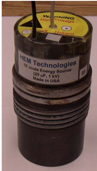
Fig. 6.10 Compact battery/capacitor powered seed source developed by HEM Technologies for small and medium FCGs. The energy density is roughly 30 \text{ mJ/cm}^3 . (Courtesy of D. Hemmert.)
