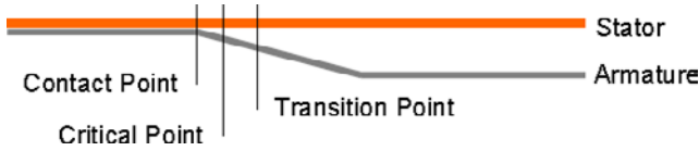
Fig. 6.4 Kiuttu and Chase divide the helical FCG into sections separated by two points: Critical Point, where the local Magnetic Reynolds Number is unity, and the Transition Point, where the wire-to-wire proximity effect is equal to the wire-to-armature proximity effect [18].
