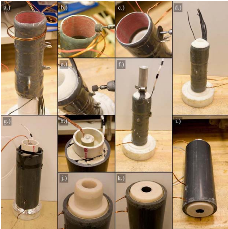
Fig. 14.13 The remaining steps in HFCG fabrication following the completion of the stator. (Courtesy of Thomas Holt and Andrew, Texas Tech University.)
