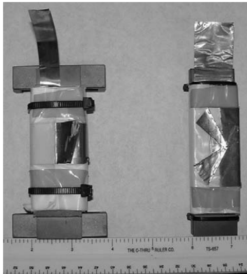
Fig. 12.38 Photograph of the VIGs used in the FEG-VIG experiments [15].
