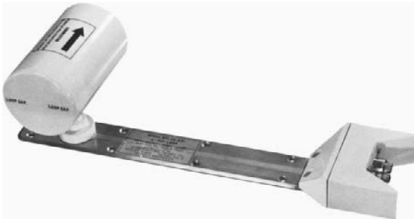
Fig. 4.15 EG&G multi-turn loop or B-dot free field sensor.
