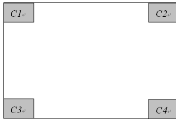
Fig. 2. Illustration of Four Corner Blocks for Judging Illumination Changes in Circumstance
