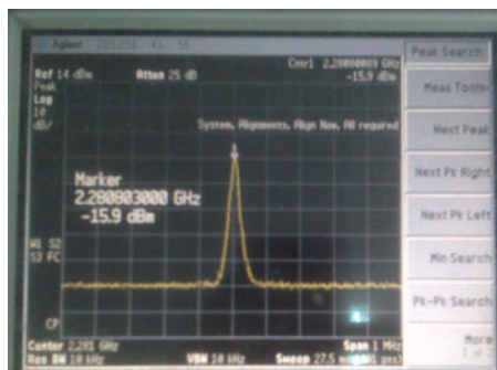
Fig. 9. Output signal of the radio beacon
