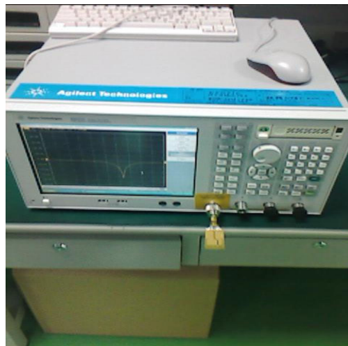
Fig. 11. Return loss ( S_{11} ) measurement of a monopole antenna with Agilent E5071C instrument.
