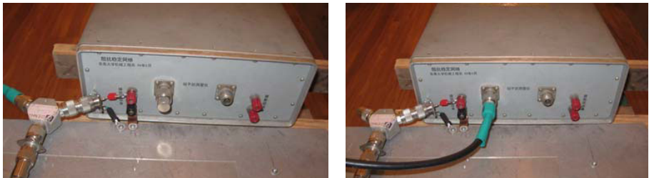
Fig. 8. Specific layouts to measure voltage division factor
