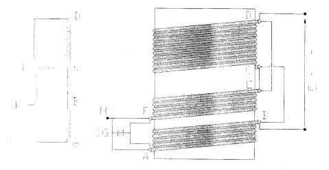
Figure 3. Winding arrangement and layout of double-Blumlein generator.
