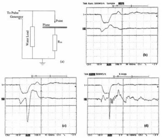
**Figure 9.** (a) Circuit diagram for streamer discharge. (b) Ch2: Signal across  $R_m = 500\Omega$  without discharge, 100V/div.; Ch1: Applied voltage pulse, 10kV/div. (c) Ch2: Signal across  $R_m = 500\Omega$  with discharge, 100V/div.; Ch1: Applied voltage pulse, 10kV/div. (d) Ch2: Signal across  $R_m = 47\Omega$  with discharge, 5V/div; Ch1: Applied voltage pulse, 10kV/div.; Time scale in (b)-(d) is 100ns/div.
