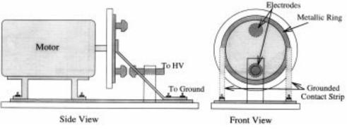
Figure 6. Schematic view of rotating spark gap switch.
