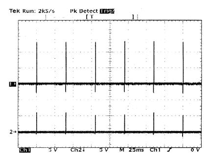
Figure 7. Oscillograph of voltage (channel 1, top trace) and current (channel 2, bottom trace) output of double-Blumlein generator with rotating spark gap.
