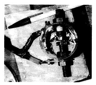
Figure 5. Spark gap switch.
