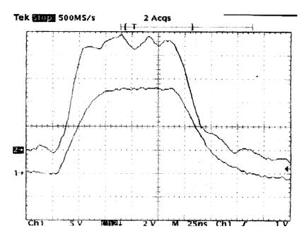
**Figure 4.** Output voltage (channel 1, bottom trace, 5kV/div; using Tektronix 75 MHz P6015A 1000X probe) and current pulse (channel 2, top trace, 20A/div; using Pearson current transformer no. 411). Time base; 25ns/div.
