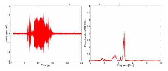
Figure 4.22 – Microwave signal and FFT of HPM system at 21 kV charging with 9 mm A-K gap.
