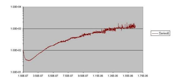
Figure C.5 – Resistance under pulse excitation as a function of time for a 150  $\Omega$  nominal resistance.
