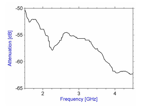
Figure F.1 - Attenuation of 10 m section of RG58 coaxial cable
