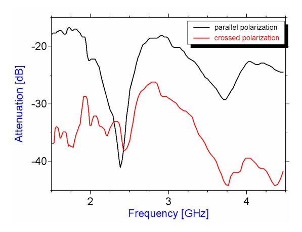
Figure F.2 - Attenuation of parallel and crossed polarization of the Horn adaptor.
