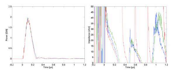
Figure 4.21 – Power and impedance of HPM system at 21 kV charging using a Vircator load with 9mm (green), 10mm (blue), and 11mm (red) AK-gap.
