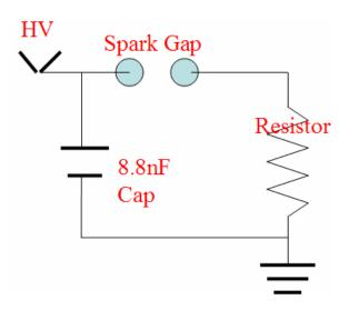
Figure C.1 - Resistor testing setup
