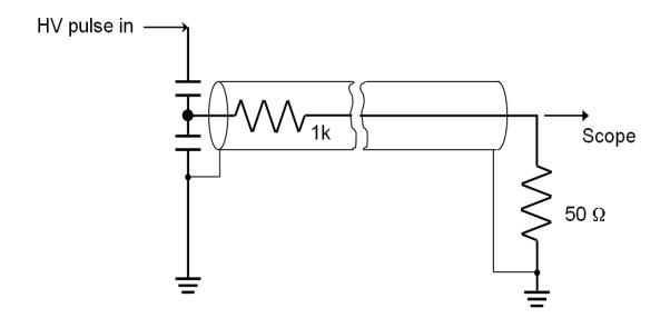
Figure 3.16 – Circuit schematic of capacitive voltage probe.
