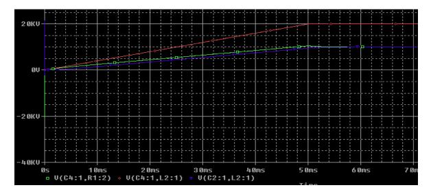
Figure 4.8 - Spark-gap design charging simulation
