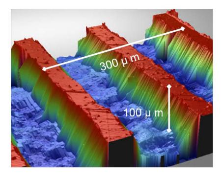
Figure 3.28 - Optical interferometer image of 100 um depth aluminum cathode
