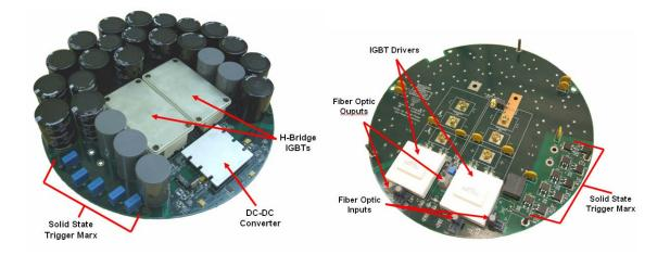
Figure 3.2 – Inverter PCB board
