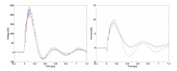
Figure 4.20 - Voltage and current of HPM system at 21 kV charging using a Vircator load with 9mm (green), 10mm (blue), and 11mm (red) AK-gap.
