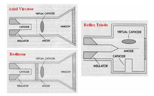
Figure 2.6 – Conceptual sketches of basic operation geometries of the Axial Vircator, Reditron, and Reflex Triode virtual cathode microwave devices [27].
