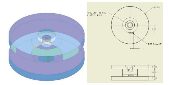
Figure 3.7 - Lexan inductor casing
