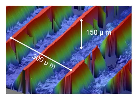
Figure 3.29 - Optical interferometer image of 150 um depth aluminum cathode
