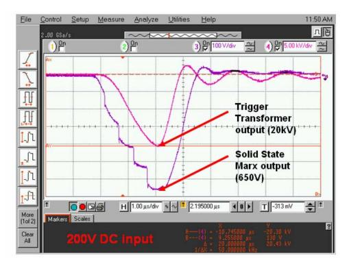
Figure 4.5 – Output of 5 stage thyristor solid state Marx and the trigger wave form after the inductor
