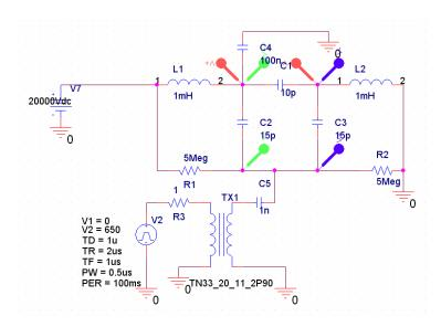
Figure 4.6 – Solid state Marx triggering simulation circuit
