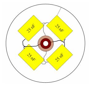
Figure 3.6 – Early capacitor setup for single Marx stage
