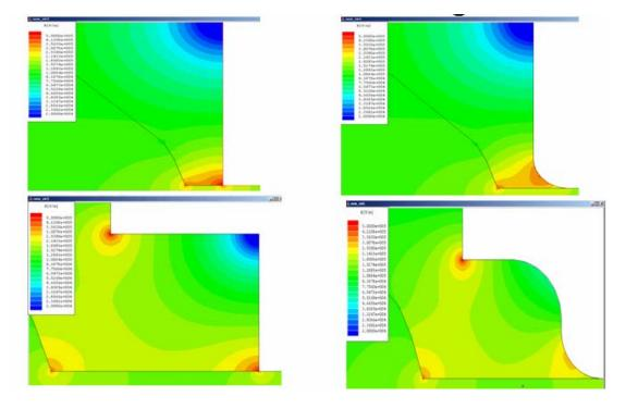
Figure D.2 - Field shaping for new connection at triple point 2 A base design for the HV feed-through is simulated in figure D.3 and some basic field shaping of the triple points in the added water resistor section seen with the protrusions of the brass piece seen in figure D.4
