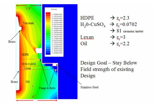
Figure D.3 - Base design of added stages
