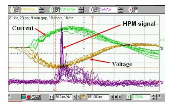
Figure 4.25 - Screen shot of diode power, voltage, and current wave-forms of a burst of 10 shots at  ${\sim}10$  Hz.
