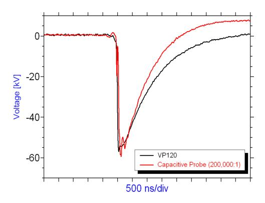
Figure 3.14 – Wave form matching between VP120 probe and the capacitive voltage probe.
