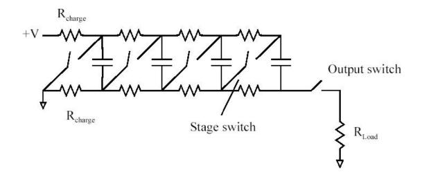
Figure 2.1 – Sample Max generator charging circuit [5].
