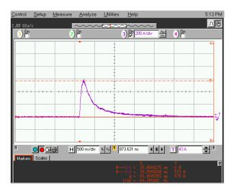
Figure C.3 - Non-linearity of Ohmite resistor
