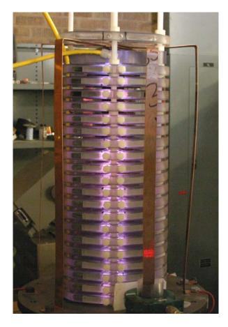
Figure 4.9 - 20 stage CMG fired into short at low charging voltages.
