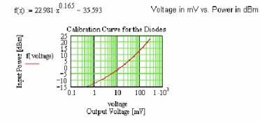
Calculation of Power delivered to diode detector from voltage measured on Oscilloscope:
