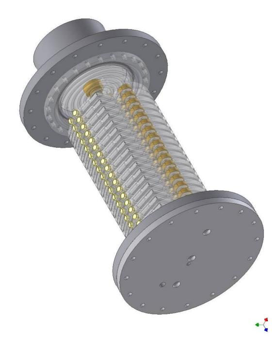
Figure 3.12 – View of 20 stage CMG without casing
