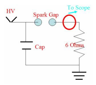
Figure 4.1 - Capacitor testing setup
