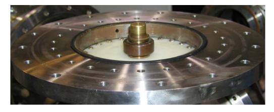
Figure 3.20 - Coaxial water load section
