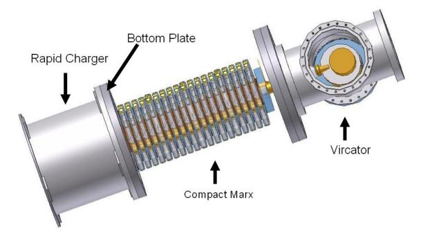
Figure 1.2 - Complete HPM system. Overall length  $\sim 150$  cm. Main diameter  $\sim 30$  cm.
