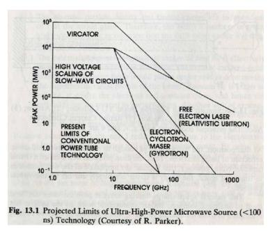
Figure 2.5 – Projected limits of Ultra-High-Power Microwave Source Technology [15]
