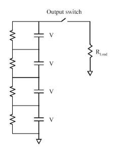
Figure 2.2 – Sample Marx generator discharging circuit [5].
