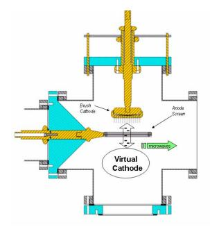
Figure 3.39 - Reflex Triode Vircator configuration
