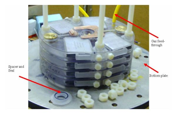
Figure 3.10 - Marx assembly with the first 4 stages
