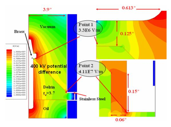
Figure 3.22 – Original Design Simulation
