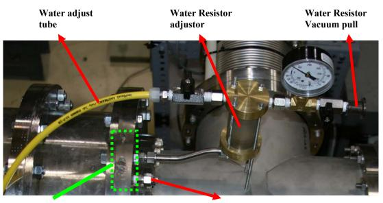
213 Ohm water resistor section
