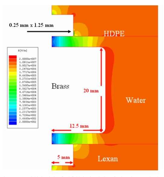
Figure 3.26 – Field simulation final field shaping design of point 3 in protection load section.
