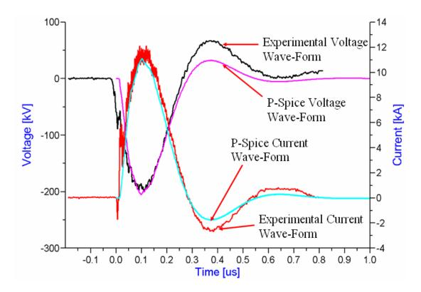
Figure 4.18 - Wave matching of Marx model at 17 kV to measured output waveform with water load of ~20 kV charging, 10 Hz shot, with rapid charger.
