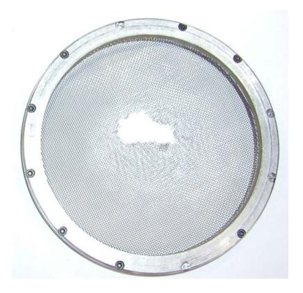
Figure 3.31 – Used screen anode constructed with steel mesh
