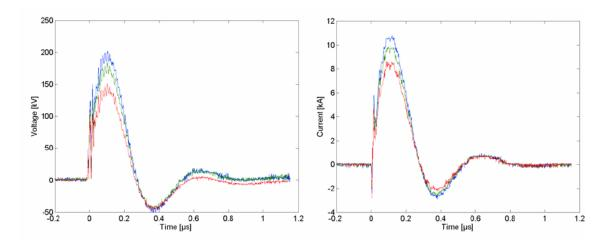
Figure 4.14 - Voltage and current of HPM system into an 18.5 Ohm water load with 15 (red), 17.5 (green), and 20 kV (blue) charging.
