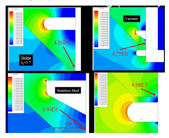
Figure D.1 - Field shaping tests for triple point 2
