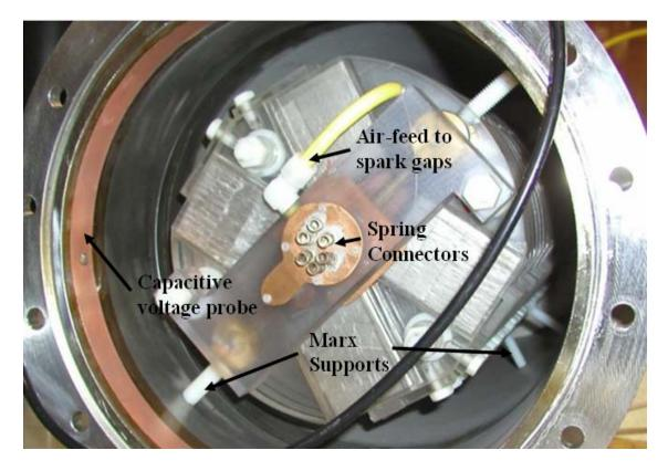
Figure 3.13 - Top stage of Marx, spring connection to HV feed-through, and 200,000:1 capacitive voltage probe.
