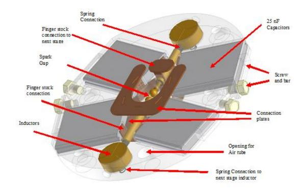
Figure 3.9 - Single stage assembly of the Compact Marx
