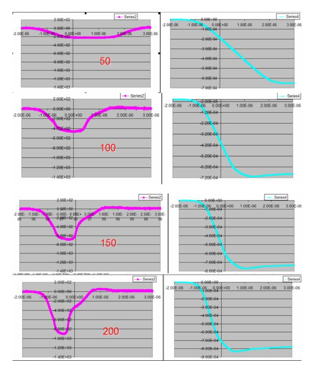
Figure C.6 – Inductor core (ETD 44-3F3, 12.5 mm diameter) testing with 10 turns on the primary, using 50, 100, 150, and 200V charging (Left column: Transformer output voltage. Right column: Volt-seconds)
