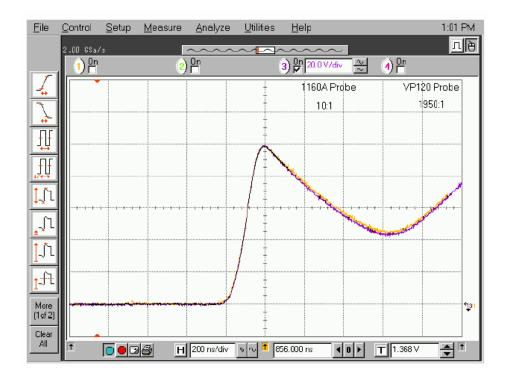
Figure 3.15 – Comparison of the VP120 and HP1160 probes.
