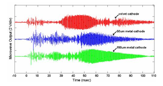
Figure 4.31 - Comparison of microwave signals of the velvet, 100 μm, and 150 μm aluminum cathodes at 6mm A-K gap [11].
