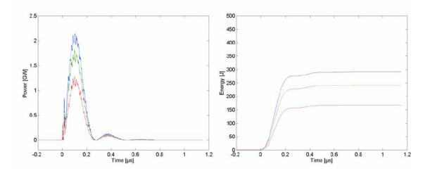
Figure 4.15 - Power and energy of HPM system into an 18.5 Ohm water load with 15, 17.5, and 20 kV charging.
