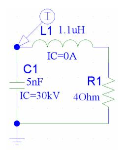
Figure 4.10 - Lumped element representation of 1.5 kV charging, 20 stage CMG into short.
