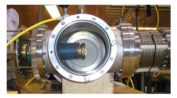
Figure 3.35 - Water load mounted in system
