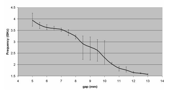
Figure 4.30 – Microwave frequency vs. gap distance of velvet cathode over 4 sets of data.
