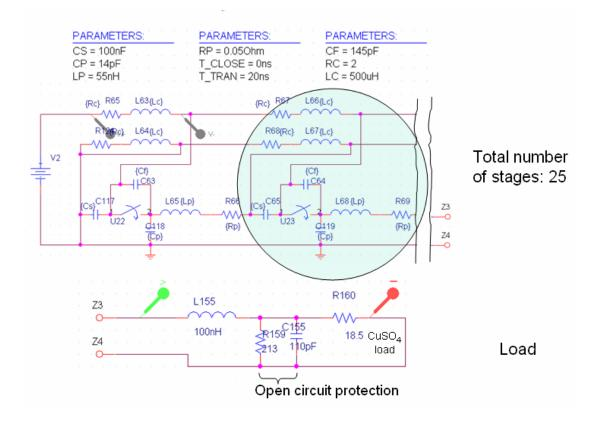
Figure 4.17 - P-spice modeling of the electrical characteristic of the full 25-stage CMG model fired into an 18.5  $\Omega$  water load
