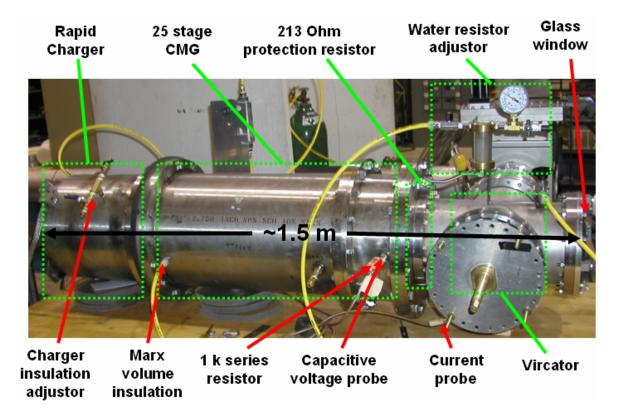
Figure 4.13 - Side view of complete HPM system
