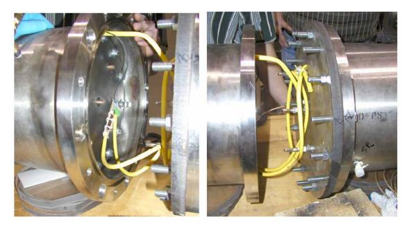
Figure 3.3 – Connection between the rapid charger and the CMG.
