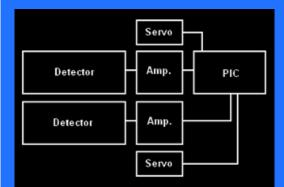
This is a simplified hook up diagram for the device. The A/D converter isn't shown.
