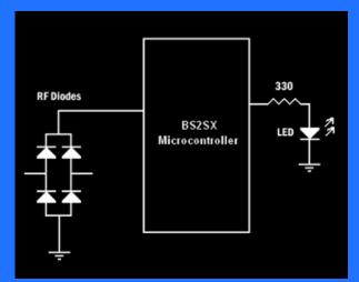
This is the simple unamplified true/false detector that senses the cell phone when the RF bridge rectifier sets the microcontroller input to high.
