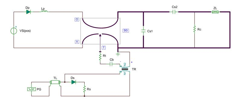
FIGURE 4. LC-inversion circuits.
