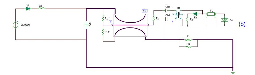
FIGURE 5. Typical series circuits using field-distortion switches.
