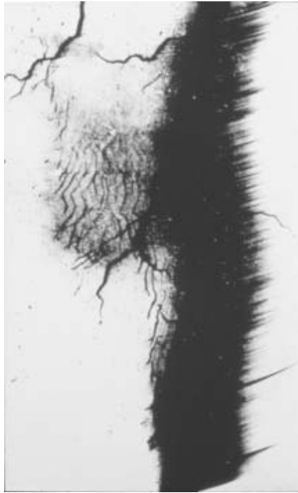
Figure 3.2 Spatial development of the negative downward flash (courtesy of 'Progressive lighting: A comparison of photographic and electrical studies of the discharge', by B.F.J. Schonland and H. Collens, Proceedings of the Royal Society. Series A , vol. 143, 1934, pp. 654–674)
