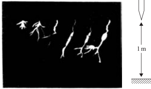
Figure 1.10 Streak photograph of development of a negative leader system, showing negative streamers ahead of the leader tip and retrograde streamers towards the anode [20]
