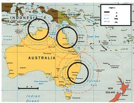
Figure 7: Endurance capabilities of the Aerosonde UAV in geographic perspective for a 2kg payload (12 hrs on station ~ black continuous circle to 0 hrs on station ~ red dotted circle)
