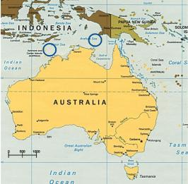
Figure 8: Typical ES sensor coverage for two areas of interest - the range estimates assume a launch from Darwin, a 2kg payload, and an altitude of 3.5km. The time on station is estimated as 15 hours.
