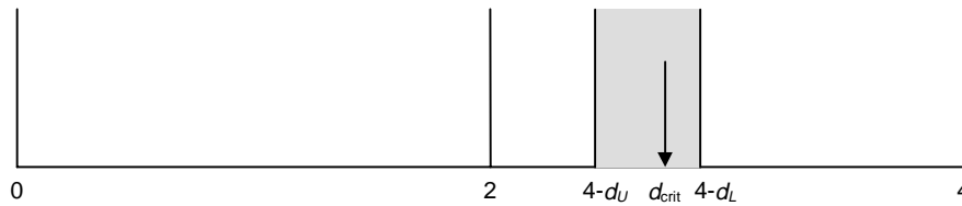
Figure 13.4. Durbin–Watson test for autocorrelation, showing the zone of indeterminacy in the case of suspected negative autocorrelation
