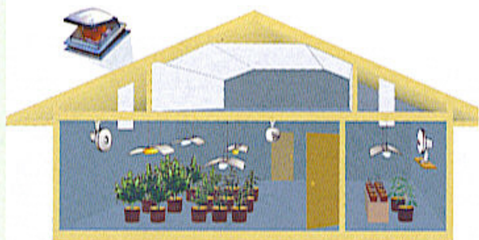
A single 1000-watt metal halide can grow enough mothers, clones, and vegetative plants to support 4000 watts of flowering HID light. This design allows pungent odors to waft upward before being evacuated via roof fans. A third area in the attic is used as a heat buffer in hot climates.
