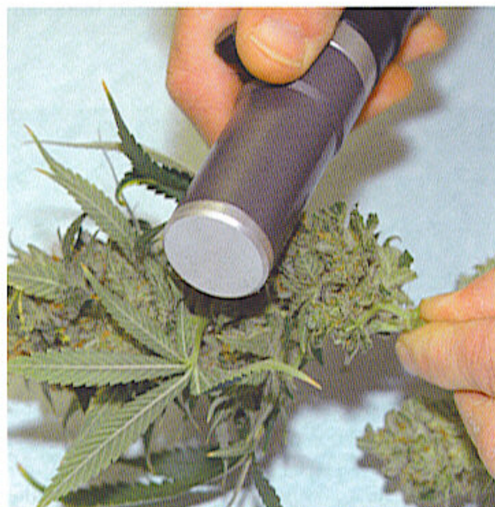
The Aardvark trimmer attaches to a vacuum which whisks all trim into a tidy bag. Put flexible hose in the freezer and shake out accumulated resin an hour later.
