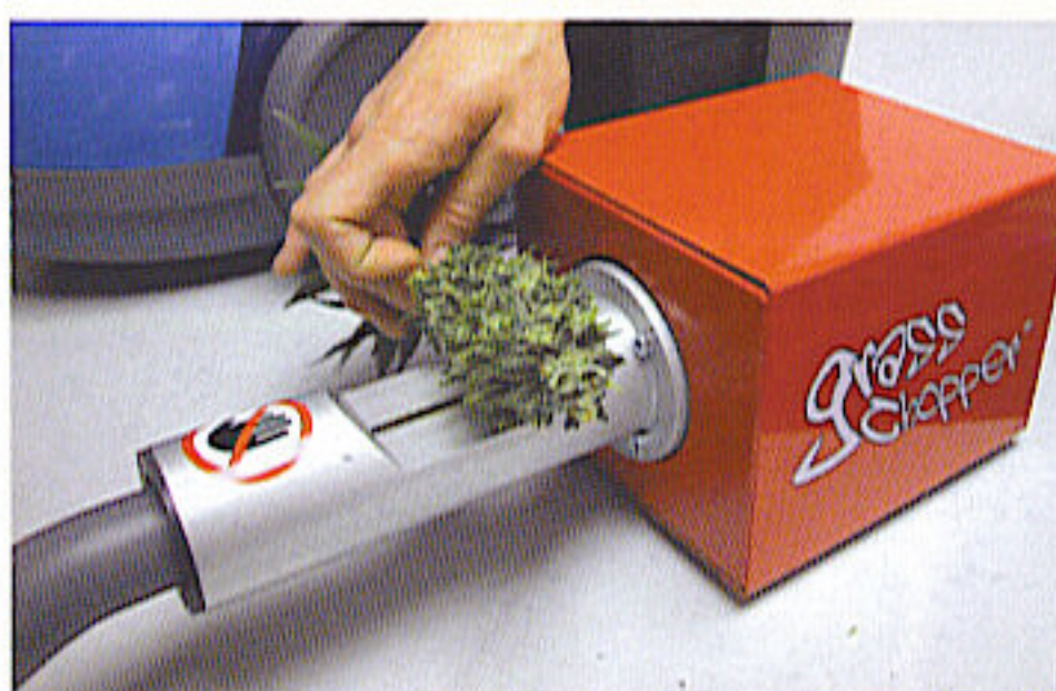
The Grass Chopper is one of the many new medium-sized bud trimmers that feature vacuum leaf removal.
