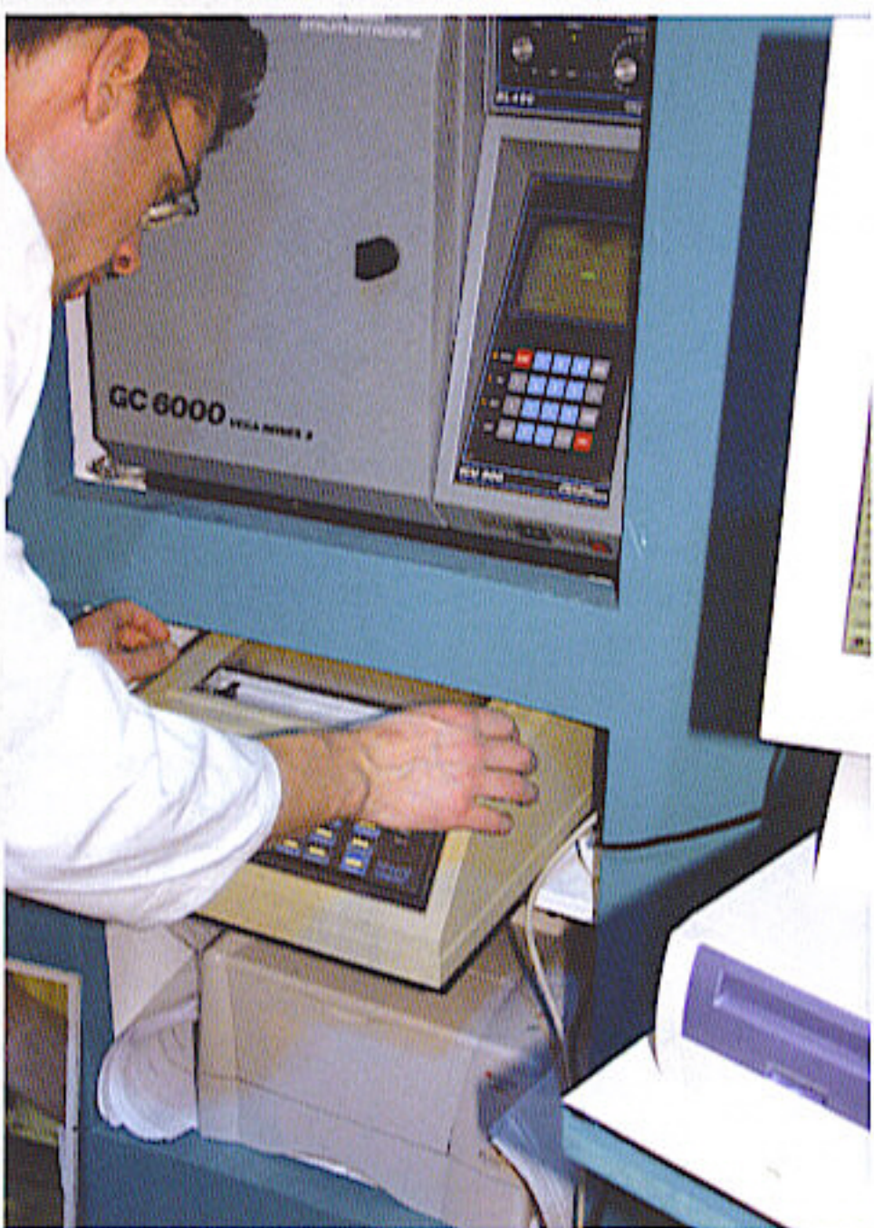
This scientist from Canna measures the exact THC content of harvested buds with a gas chromatograph.
