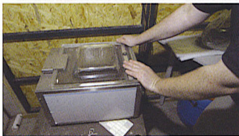
Once in place, air is removed and the bag of buds is hermetically sealed.
