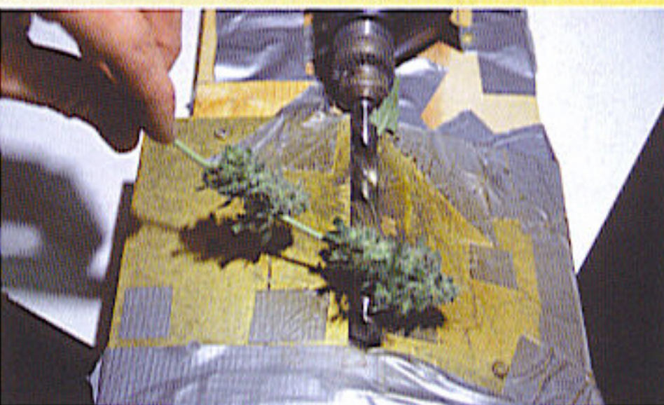
This ingenious grower made a bud trimmer by duct taping a couple of pieces of metal and a drill to a workbench.
