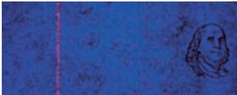
above is the “bottom” half of the paper embedded with watermark portrait and security thread Shown under black-light.
