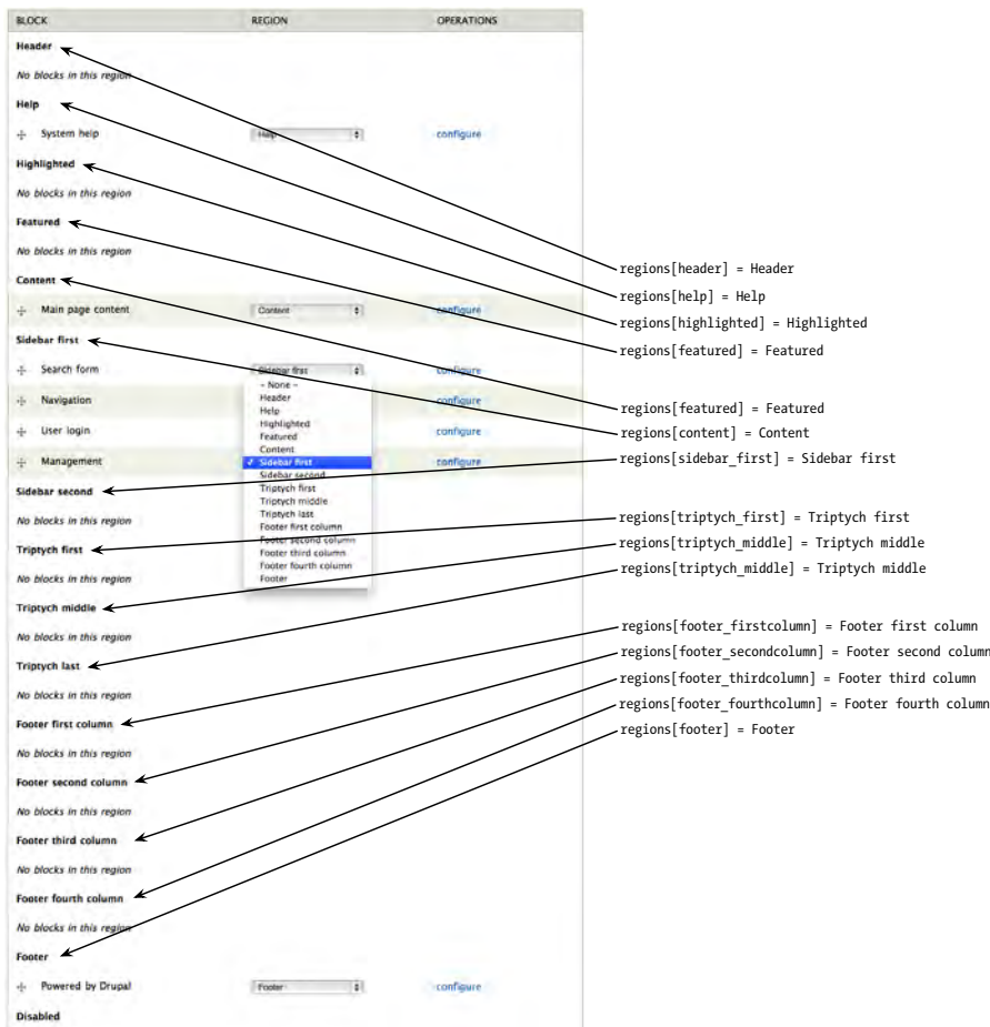
Figure 15–8. The Bartik theme’s regions and block placement options on the Blocks administration page
