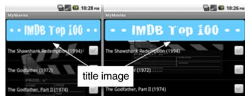
Figure 4.12 The MyMovies header image shown in portrait (left) and landscape (right) modes. In portrait mode, the image won't stretch; in landscape mode it'll stretch to fill the view horizontally, resulting in distorted proportions.
