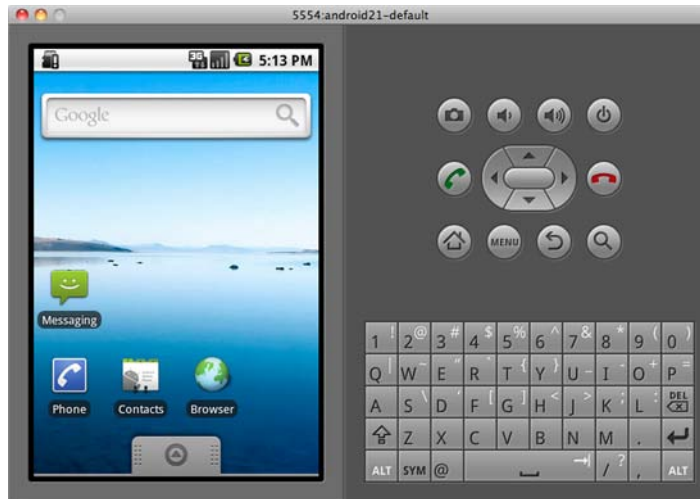
Figure 1.13 The Android emulator running an AVD image configured to work with version 2.1 of the Android platform
