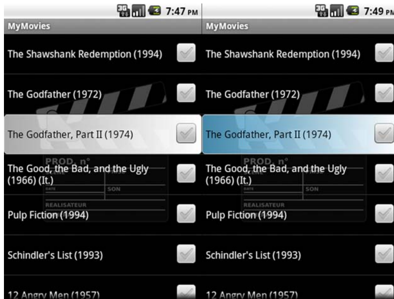
Figure 4.11 The new list selector in the default (left) and pressed (right) states. Note how it changes colors when in the pressed state.
