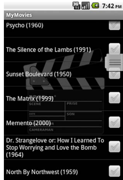
Figure 4.9 The MyMovies title screen after some styling has been applied. Note how we included a transparent background image and added a fast scrolling handle.
