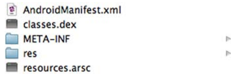
Figure 14.2 APK files are ordinary ZIP files. Uncompressing them yields a directory structure like the one above.
