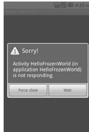
Figure 6.1 If an application becomes unresponsive (for example because it's performing expensive operations on the main application thread), Android will kill it after a few seconds and raise an exception to the user.
