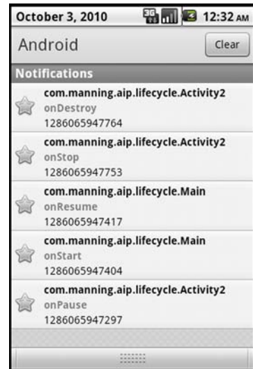
Figure 3.7 Pressing the Back key displays the lifecycle events when navigating from Activity2 back to Main .
