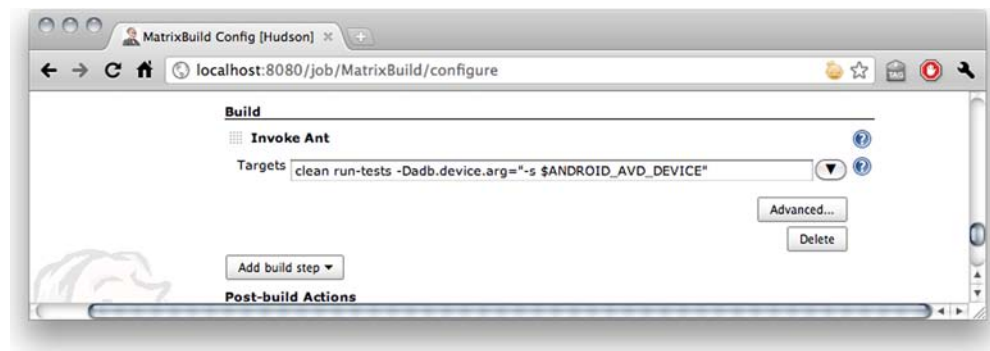
Figure 14.20 For the Ant invocation to work, we must make the specific emulator that runs the current matrix configuration available through a variable. The Android emulator plugin exports the emulator's serial number through the ANDROID_AVD_DEVICE variable, which can be passed to Ant's internal ADB task using the adb.device.arg property.
