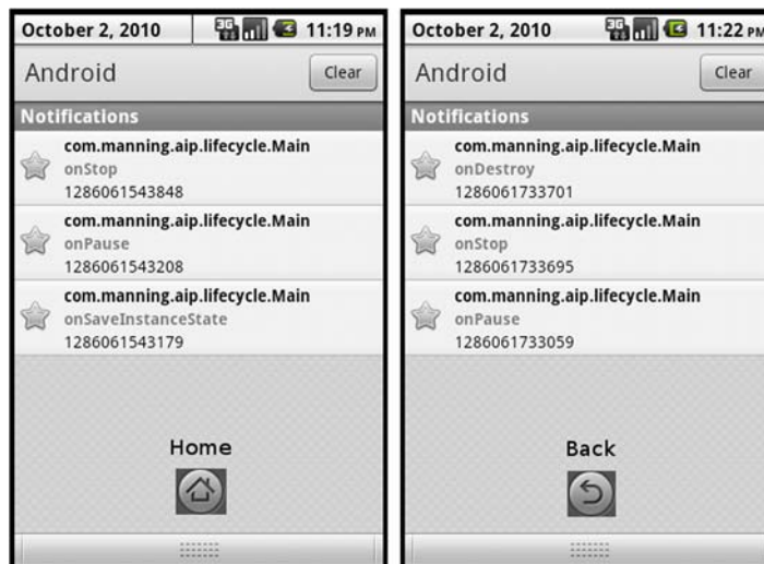
Figure 3.5 The lifecycle methods fired when pressing the Home and Back keys respectively.
