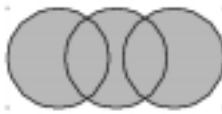
Fills based on winding—All paths are of the same direction in this example, so overlapping sections are filled.
