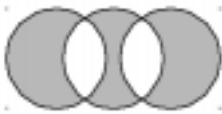
Fills based on Even/odd fill—Paths are filled and transparent regardless of direction.
