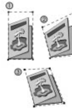
Graphics 2 and 3 show one-point and two-point perspective applied to the object in graphic 1.
