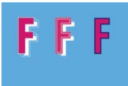
Examples of image trap placement (from left to right): spread, choke, and trapped object.
