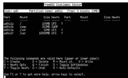
FIGURE 2.5 BSD partitions created in the partition table.
