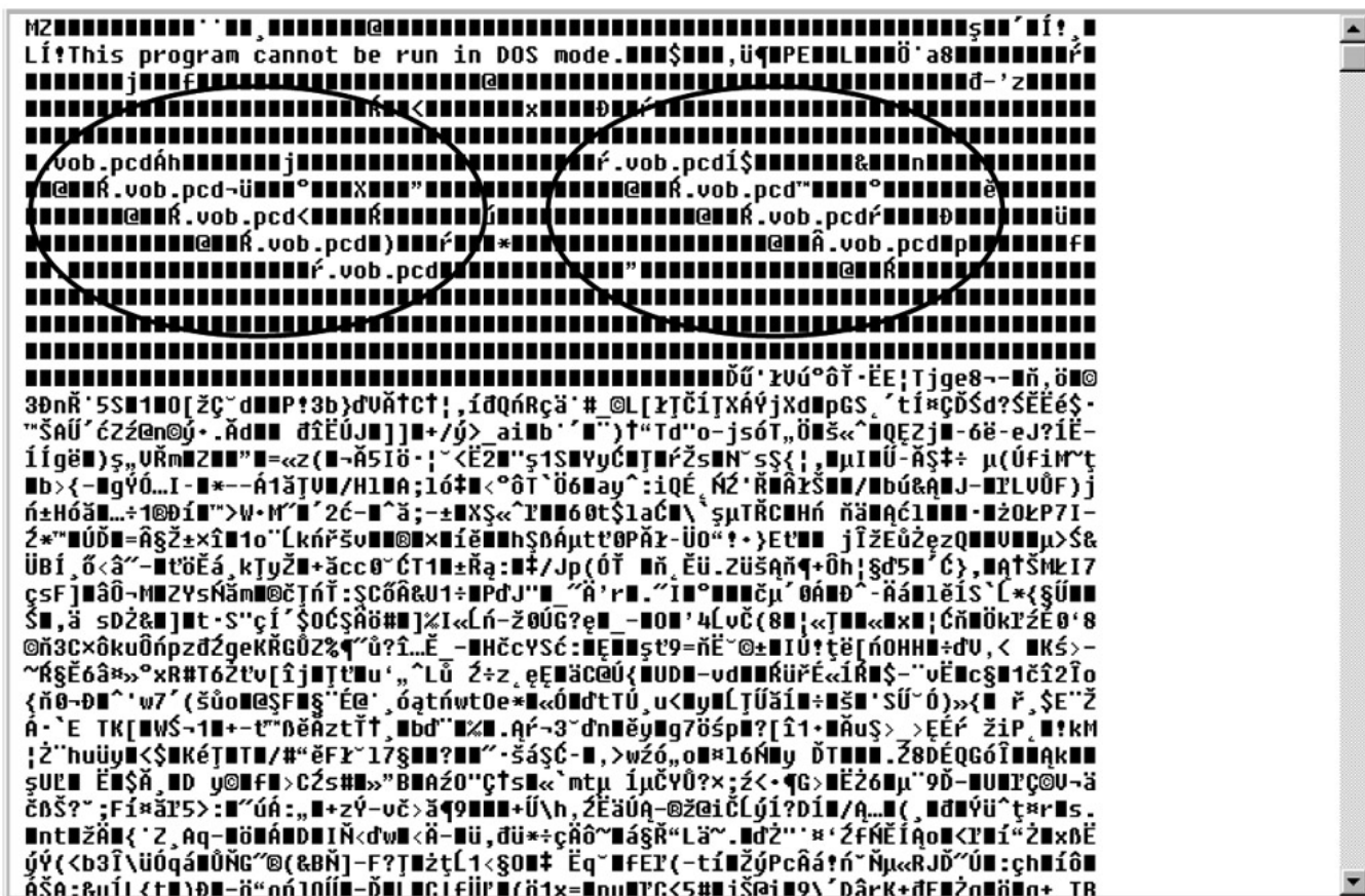
Figure 4.2: VOB is given away by the section name in the PE file header As is common with this type of protection, the program checks for errors on the original CD, which differ on copies. Decoding values for a given product are calculated according to a certain algorithm, and these values are then used to decode the original PE file. Since this is really nothing new, crackers who have managed to remove SafeDisc find it easy to remove VOB as well (see Figure 4.3).
