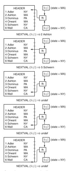
FIGURE 4.2 Interference between two query handles.
