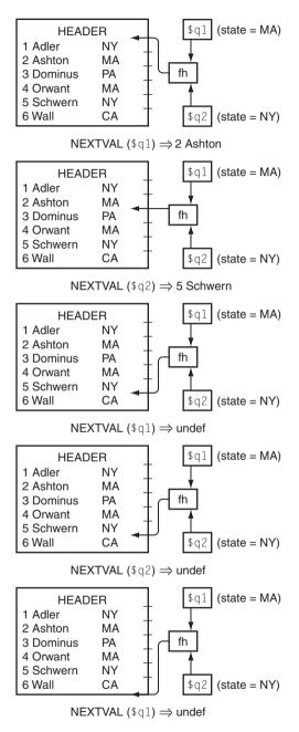
FIGURE 4.2 Interference between two query handles.
