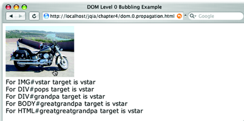
Figure 4.2 The console messages clearly show the propagation of the event as it bubbles up the DOM tree from the target element to the tree root.
