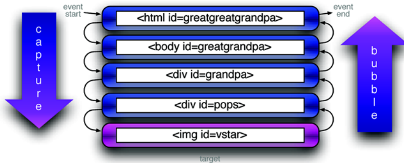
Figure 4.4 Propagation in the DOM Level 2 Event Model traverses the DOM hierarchy twice: once from top to target during capture phase and once from target to top during bubble phase.
