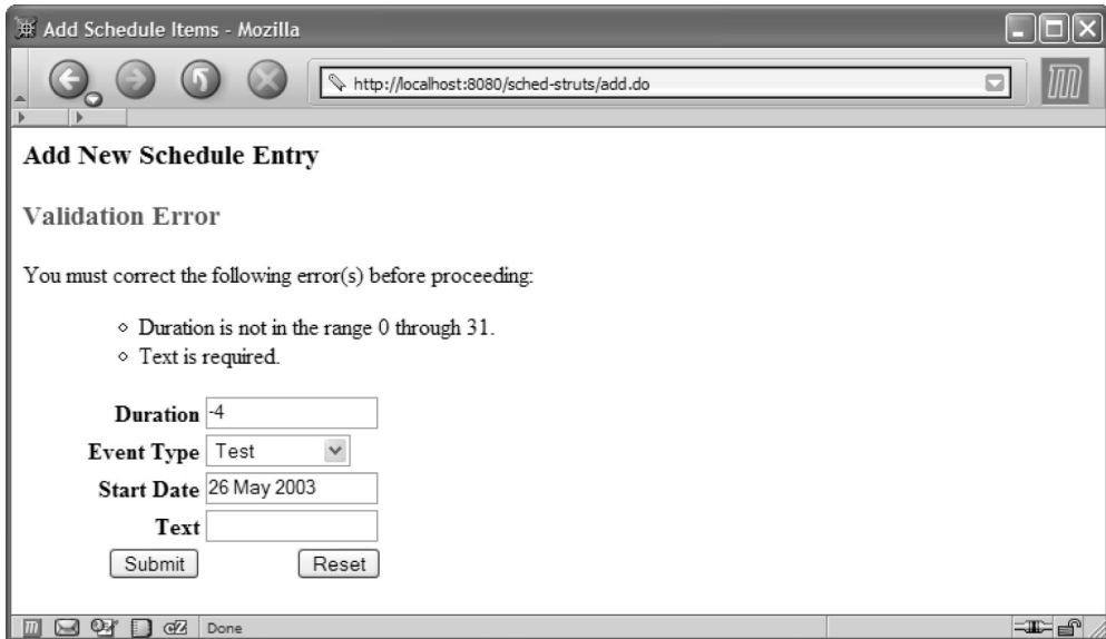
Figure 5.3 The validation in the Struts 1.1 version of the schedule application uses validations declared in the validations.xml configuration file.
