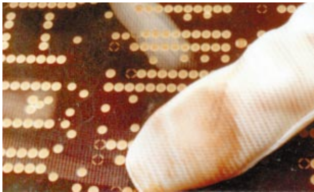
Figure 12-3 Loose black oxide crystals
