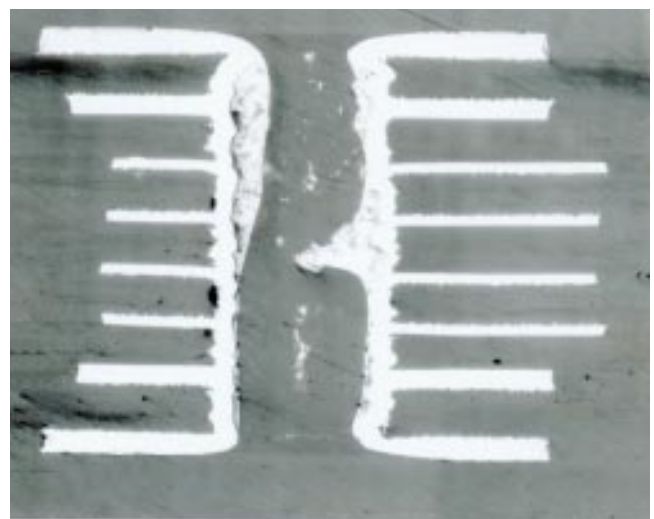
Figure 7-4 Rough hole wall due to poor drilling
