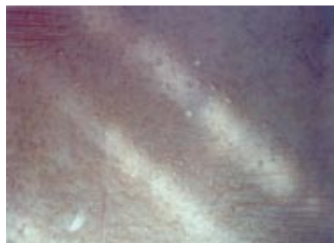
Figure 4-5 Scratches on copper treatment.
