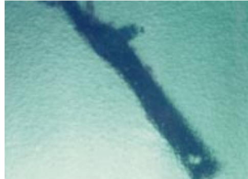
Figure 4-3. Dark spots within laminate.
