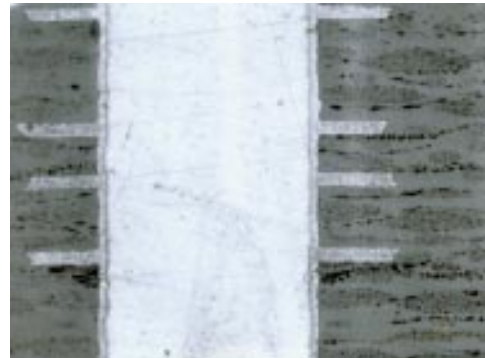
Figure 20-4. Scratches on mount surface.
