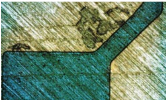
Figure 9-1 Resist scum on panels
