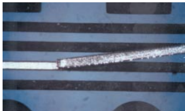
Figure 9-7 Copper-to-copper peelers after pattern plating
