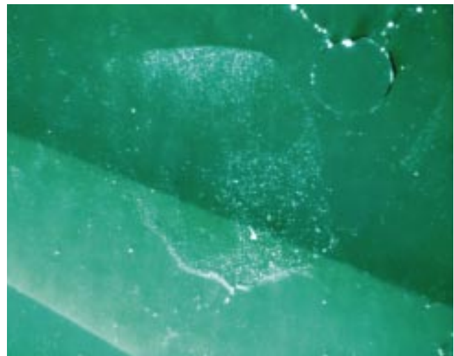
Figure 15-7 White residues on solder resist
