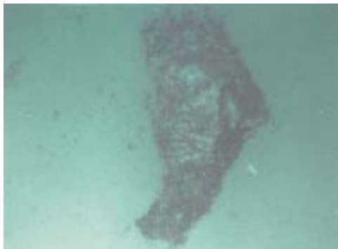
Figure 4-1. Copper or zinc inclusion in laminate.
