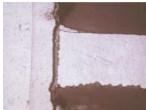
Figure 20-6. Innerlayer pull-away from barrel.
