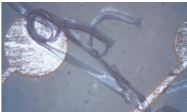
Figure 9-9 Photoresist residue on board
