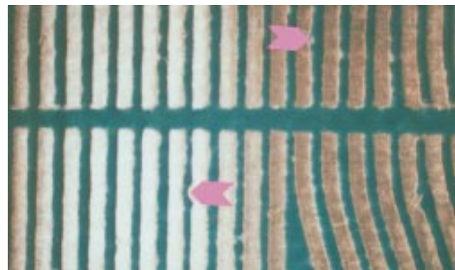
Figure 9-22 Ragged line definition
