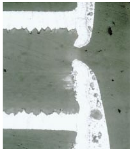
Figure 7-1 Void in hole
