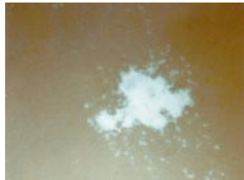
Figure 4-2. Etch pits in laminate.
