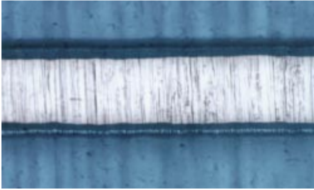
Figure 9-3 Line width reduction from incomplete development
