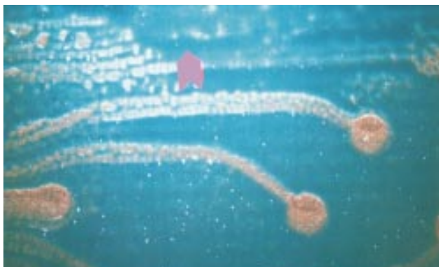
Figure 9-17 Ink runs through screen
