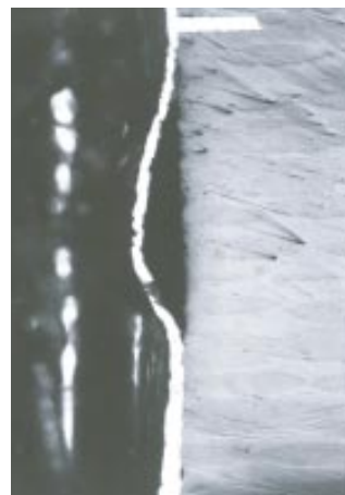
Figure 20-2. Plating torn away during microsection preparation because of potting compound void in hole.
