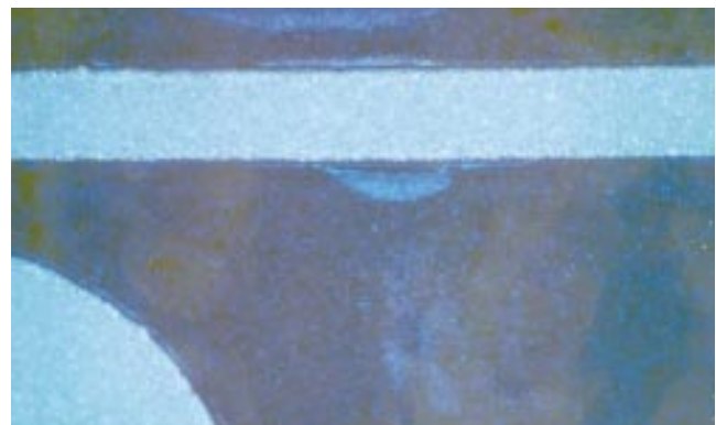
Figure 9-11 Resist breakdown during pattern plating
