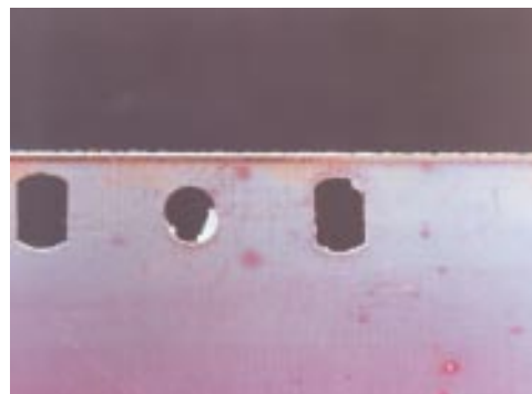
Figure 5-7 Rough edges of punched hole
