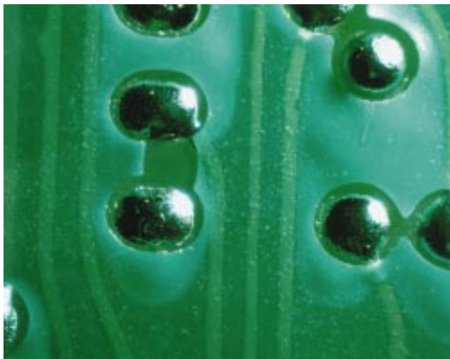
Figure 15-6 Solder resist breakdown
