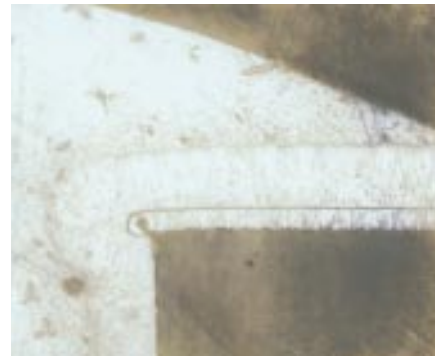
Figure 5-6 Connected curl chip
