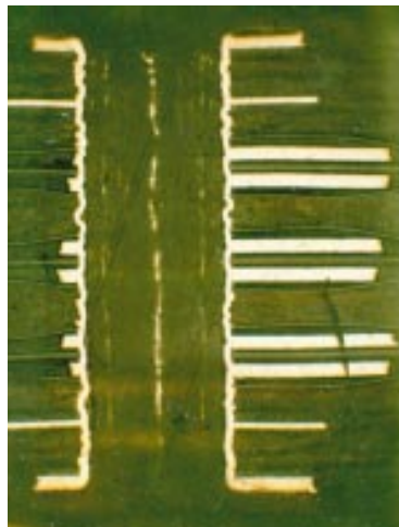
Figure 13-1. Misregistration of innerlayers as evidenced by shifted lands.
