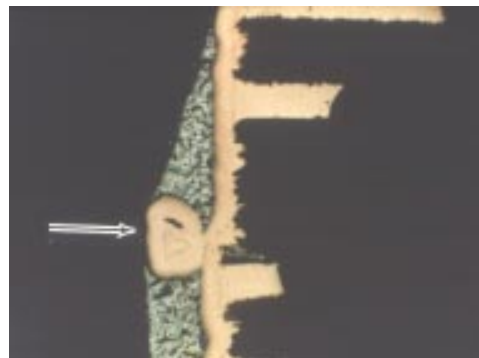
Figure 10-1. Nodules from copper plating.
