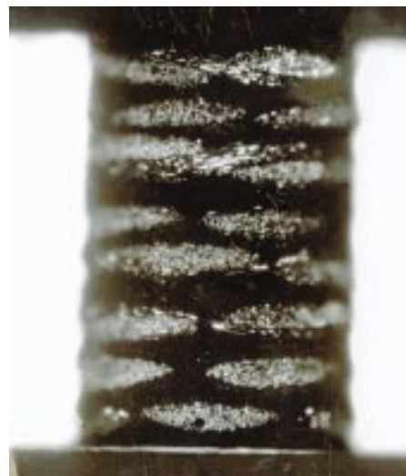
Figure 7-2 Glass voiding as seen using backlighting technique
