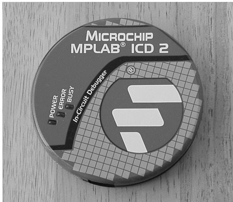
Photo 5.2: This is the MPLAB ICD 2; otherwise known as the hockey puck. The MPLAB ICD 2 uses debug facilities built into the PIC18F452 to give us a marvelous view of the PIC18F452's internals.
