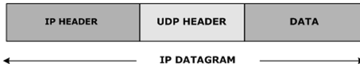
Figure 10.1: There are 28 bytes of header information in the UDP datagram. The UDP datagram is riding inside the IP datagram, which will all ride in the Ethernet frame.
