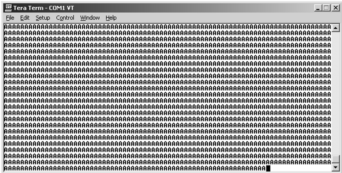
Figure 2.9: Notice I “paced” the transmission in Code Snippet 2.4. After the first ‘A’ was sent, each ‘A’ thereafter was sent one per second (delay_ms(1000)).
