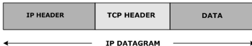
Figure 11.1: Let's count 'em up...20 bytes for the IP header, and 20 more for the TCP header. Remember what you learned about encapsulation and UDP? You'll need that again for TCP.
