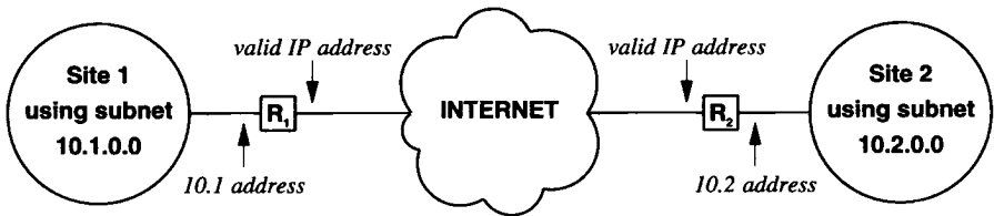
Figure 20.4 Illustration of addressing for a VPN that interconnects two completely private sites over the global Internet. Computers at each site use private addresses.
