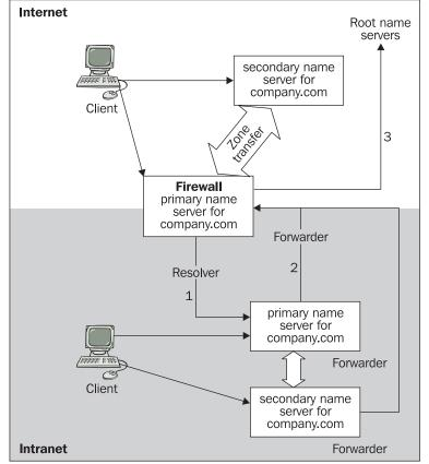
Figure 10.3: Company DNS zone is divided into two independent zones with the same domain name company.com, but with a different content
