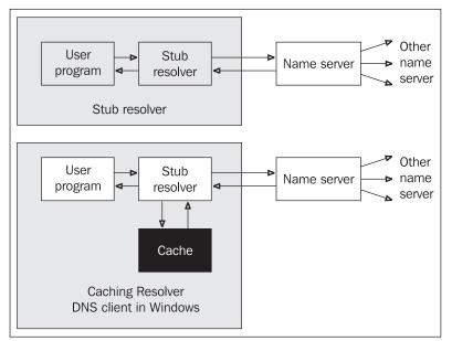
Figure 1.5: Stub resolvers and caching resolvers
