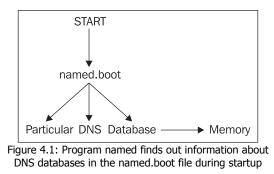
A DNS database consists of individual files that are specified as the last parameters of the individual commands of the named.boot configuration file. A database on a disk may contain the following types of data:
