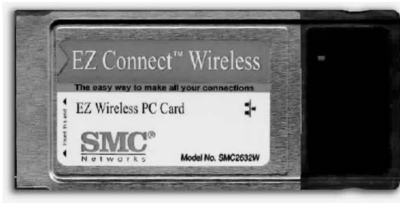
Figure 8.15 The SMC networks EZ wireless PC card is designed for insertion into a Type II PC slot in a notebook or laptop computer.
