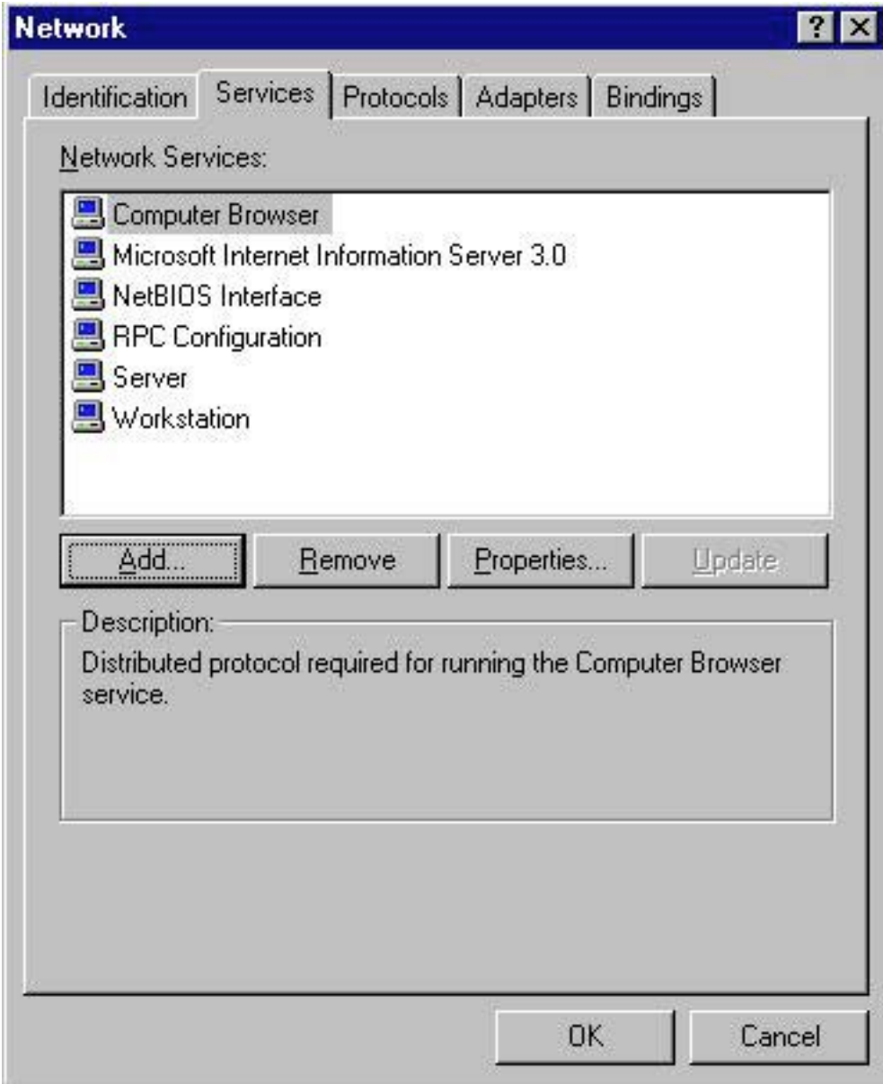
Exhibit 9.3. Installing Remote Access Services on an NT Server Requiring Selection of Services Tab from the Network Dialog Box
