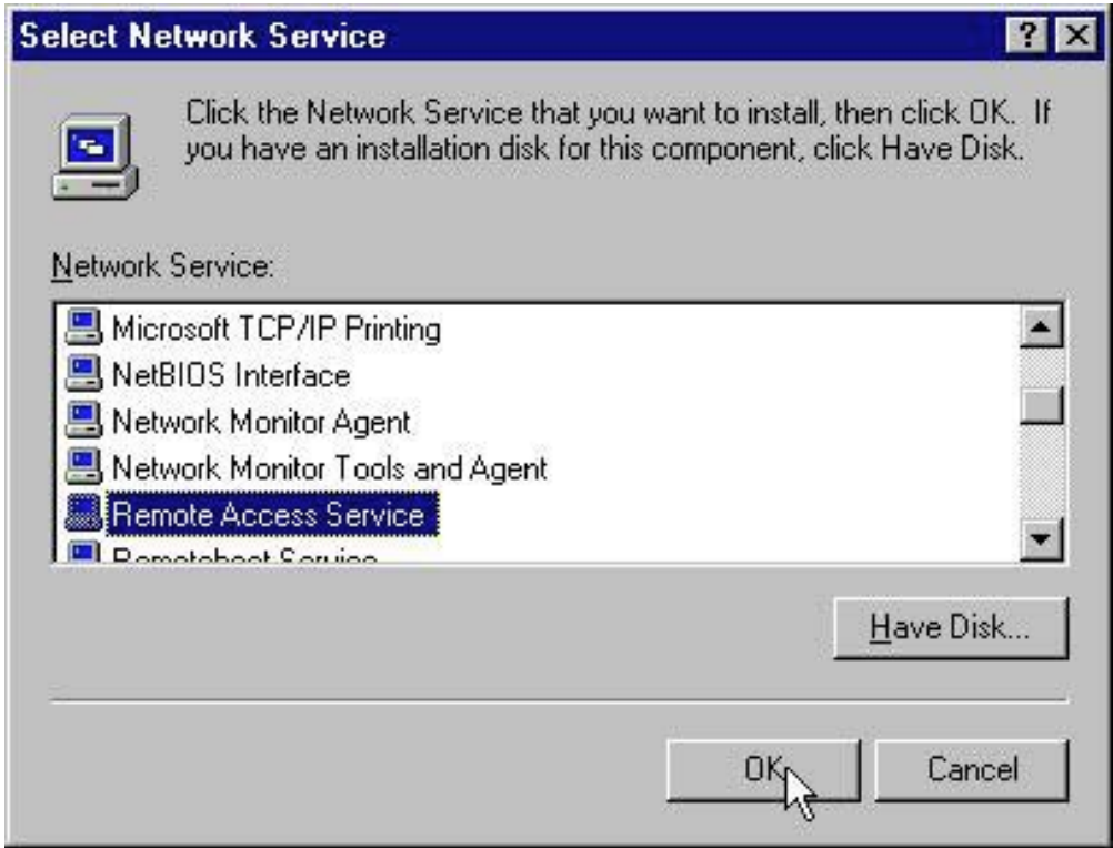
Exhibit 9.4. Installing RAS from the Select Network Service Dialog Box
