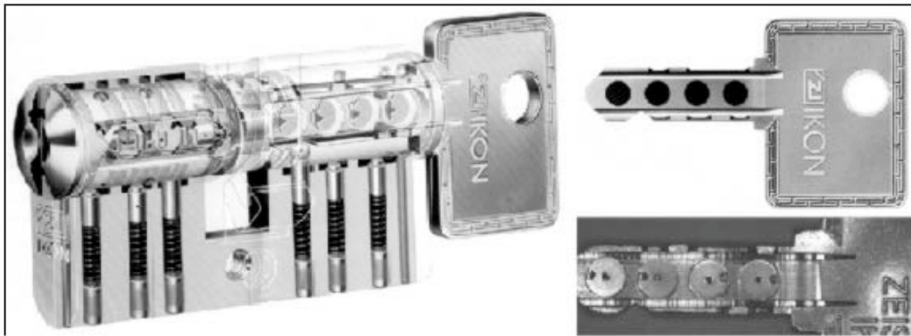
Figure 19-08. The Ikon magnetic lock is one of the most secure in the world. The mechanism is comprised of eight rotating magnetic discs that control two sidebars, as well as secondary pin tumblers. If all of the discs are not in alignment, the sidebars are not able to retract, thus preventing plug rotation. Courtesy Ikon.
