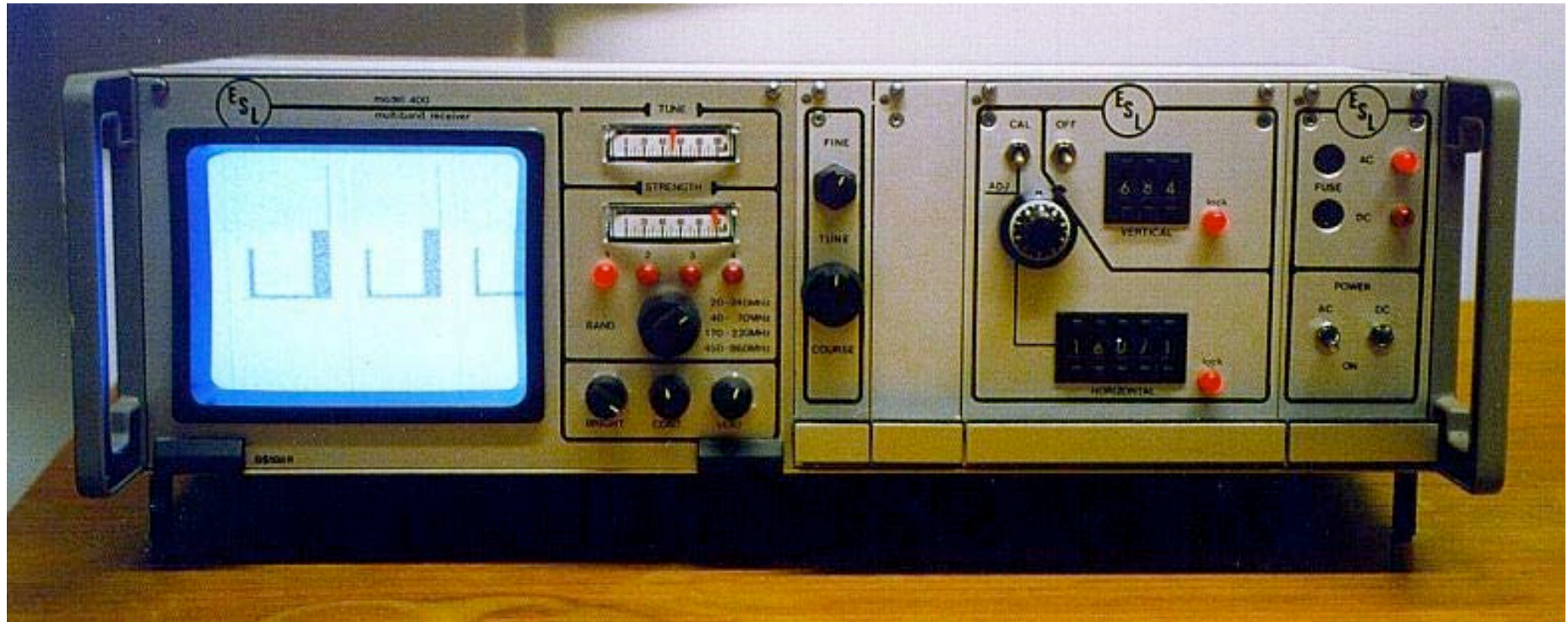
DataSafe/ESL Model 400 Tempest Emission Monitor
