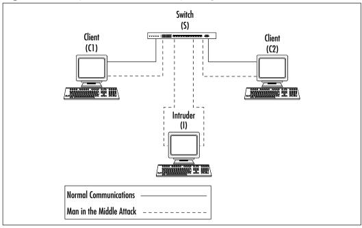
Figure 6.4 Sample Network for ARP Spoofing
