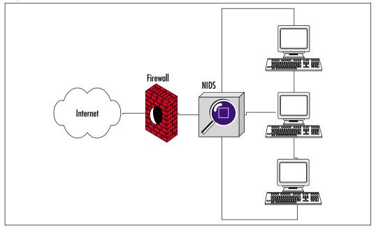
Figure 6.11 Network Intrusion Detection System
