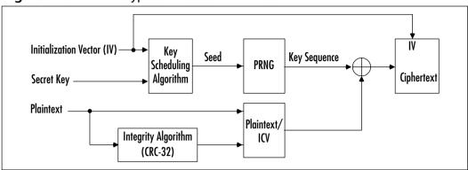
Figure 4.5 WEP Encryption Process in IEEE 802.11
