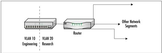
Each VLAN functions like a separate switch due to the combination of hardware and software features built into the switch itself. Thus, the switch must be capable of supporting VLANs in order to use them. The following are typical characteristics of VLANs when implemented on a network:
