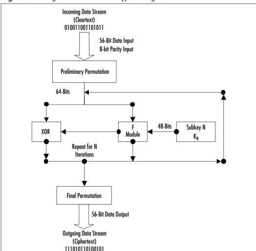
Figure 9.1 Diagram of the DES Encryption Algorithm
