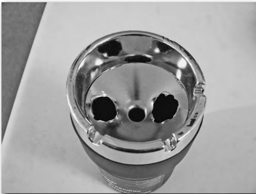
FIGURE 14-12: The holes cut in the Ash Grabber lid
