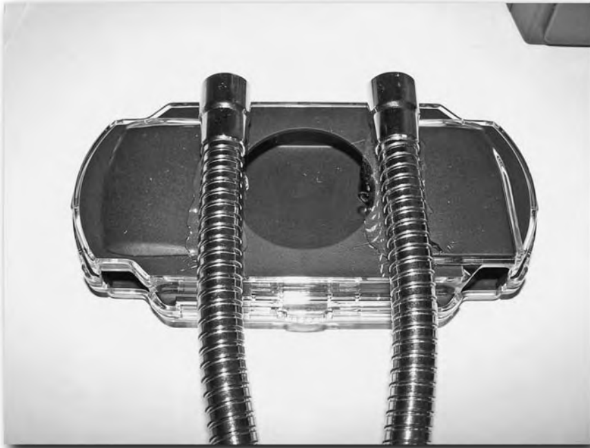
FIGURE 14-20: The extensions aligned and applied to the epoxy
