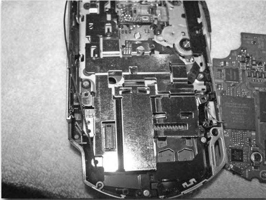
FIGURE 4-15: The screws holding the Wi-Fi card in place
