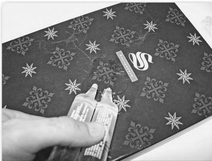
FIGURE 14-18: Mixing the epoxy
