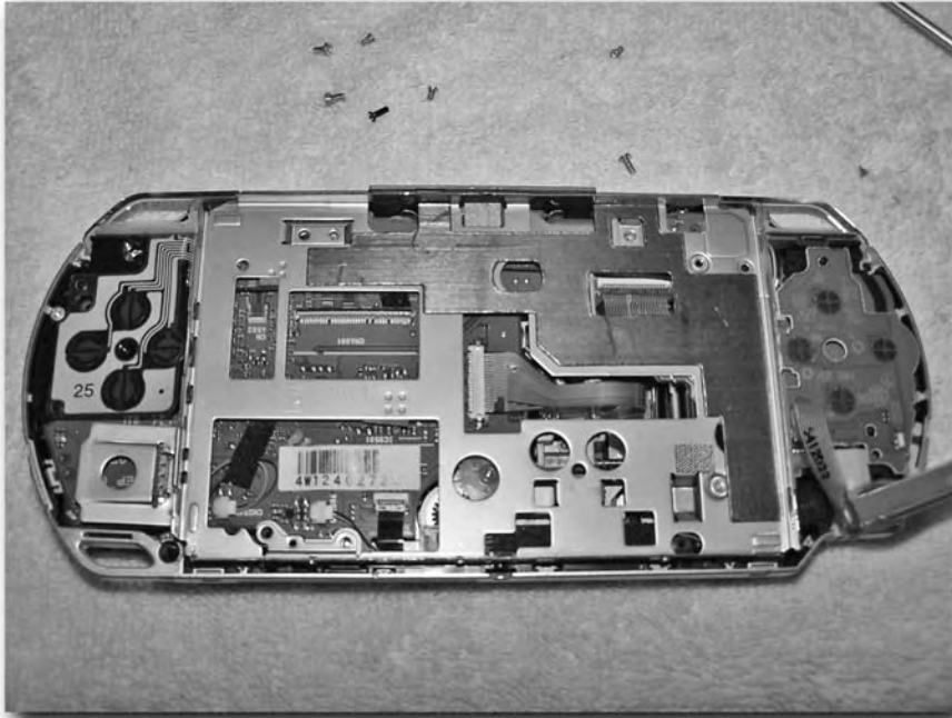
FIGURE 4-11: The metal screen holder with the nine screws removed
