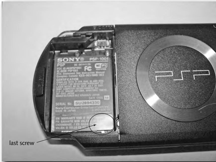
FIGURE 4-5: The last screw hides under a warranty-voiding sticker
