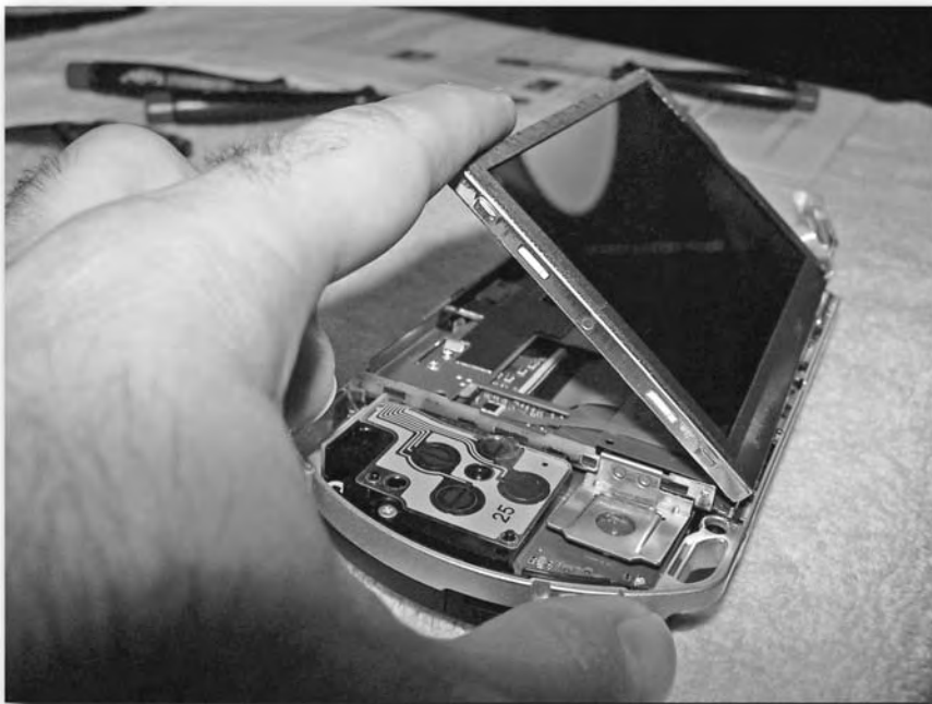
FIGURE 4-9: The screen partially removed
