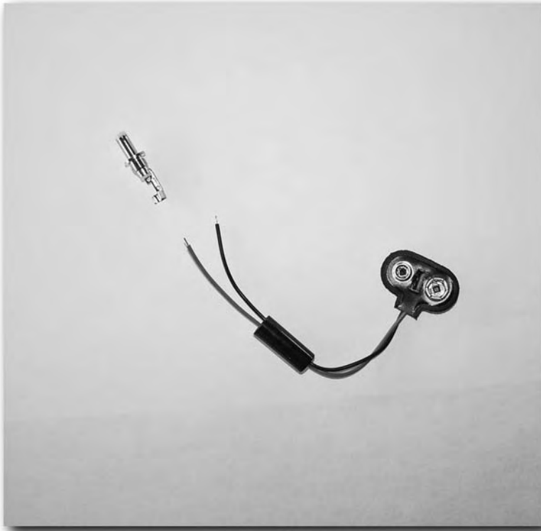
FIGURE 13-10: The snap connector wires run through the DC power plug's casing
