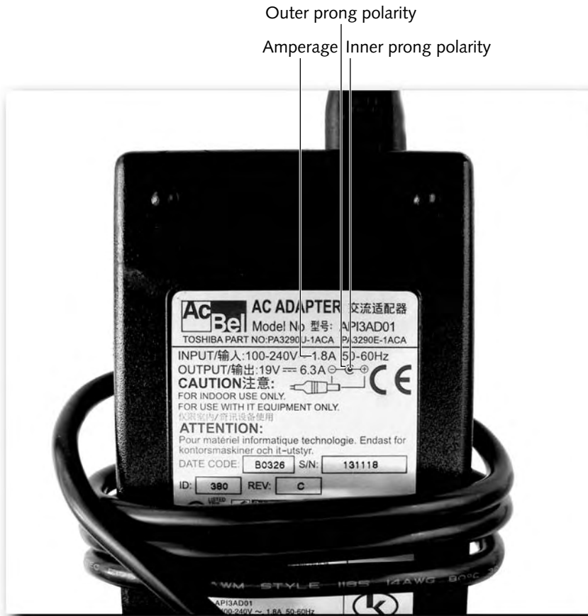
FIGURE B-1: Determining the polarity of a power supply
