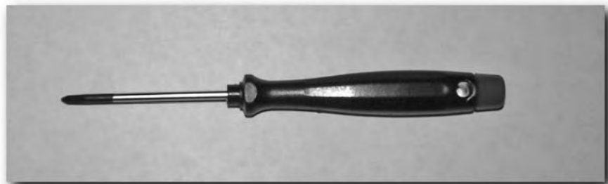
FIGURE 4-2: The precision Philips head screwdriver with a thin shaft
