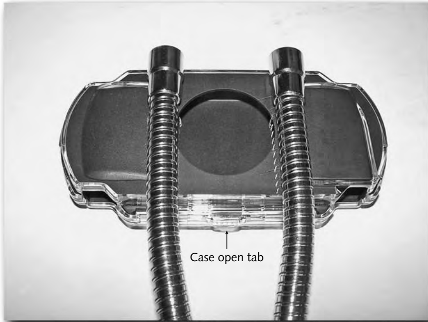
FIGURE 14-17: Make sure the case opening tab is facing you
