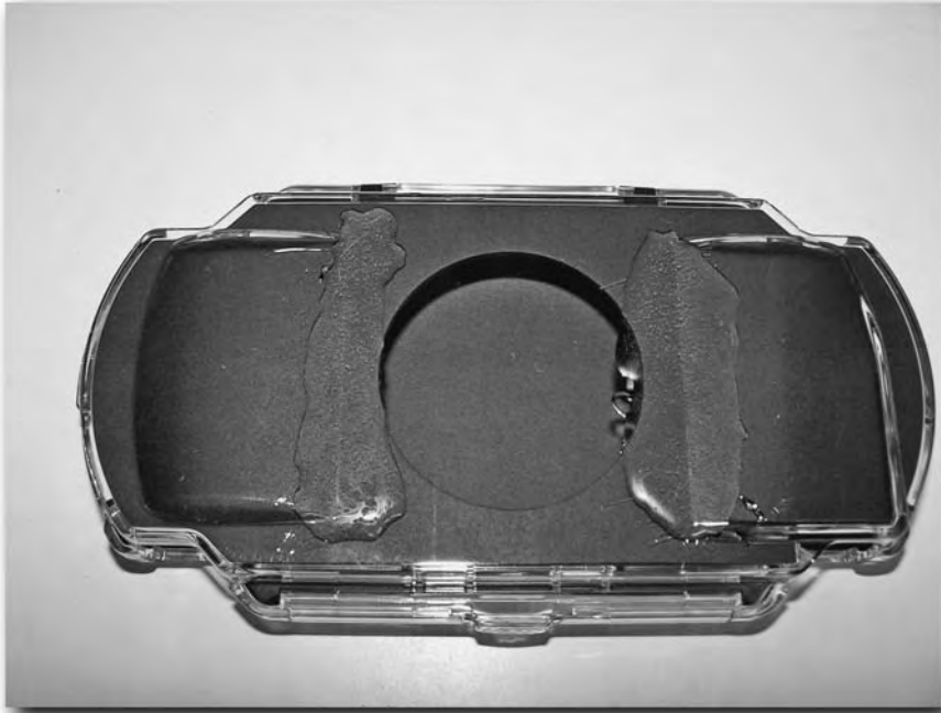
FIGURE 14-19: Applying the epoxy
