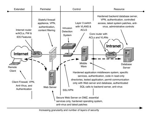
FIGURE 4.1 Defense-in-Depth within a Security Architecture
