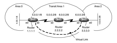
FIGURE 4.3 OSPF Network Design Example Configuration
