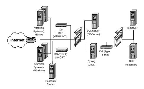
**FIGURE 8.1** Example Attacking Network
