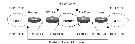
FIGURE 4.4 VPN and GRE Used to Protect OSPF Protocols over the Internet
