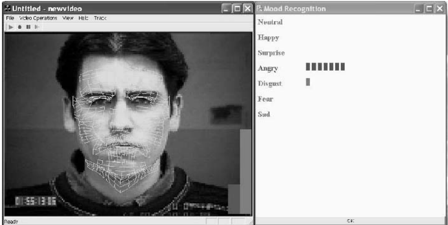
Figure 10.2. A snap shot of our realtime facial expression recognition system. On the right side is a wireframe model overlaid on a face being tracked. On the left side the correct expression, Angry, is detected (the bars show the relative probability of Angry compared to the other expressions). The subject shown is from the Cohn-Kanade database [Kanade et al., 2000].
