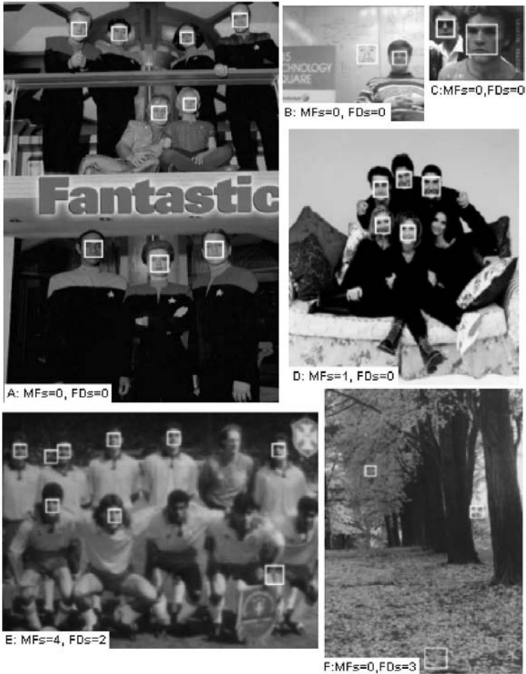
Figure 11.5. Output of the system on some images of the CMU test using the SSS classifier learned with 19,000 labeled data. MFs represents the number of missed faces and FDs is the number of false detections.
