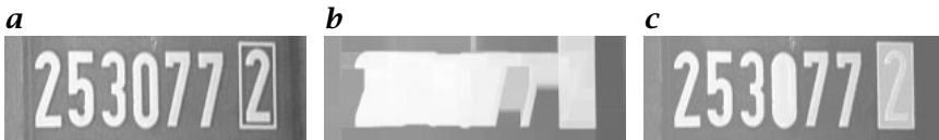
Figure 21.17: Morphological closing and closing by reconstruction of an image of a container plate: a Image of a container plate f ; b Closing of f by a 15 \times 15 square; c Closing by reconstruction of f with the same square.
