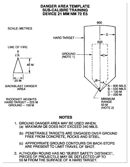
Figure 5-6 Danger area template sub-calibre training device 21 mm NM 72 E5
