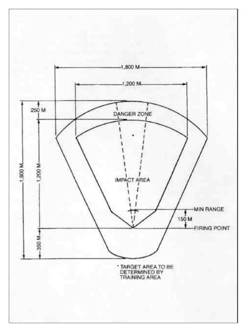
Figure 5-4 Danger Area Template - NM 72 E5, Moving Target
