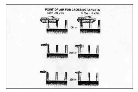
Figure 2-2-3 Point of aim for crossing targets
