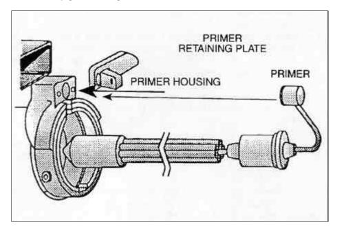
Figure 2-4-3 Loading the 21 mm sub-calibre rocket
