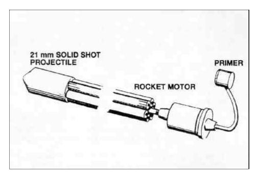
Figure 2-4-1 The 21 mm Sub-Calibre Rocket
