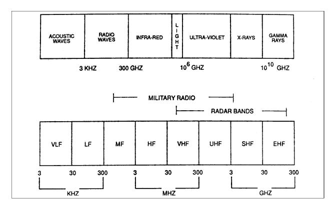
Figure 1-1-1 The Electromagnetic Spectrum
