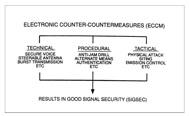
Figure 4-1-1 Electronic Counter-Countermeasures
