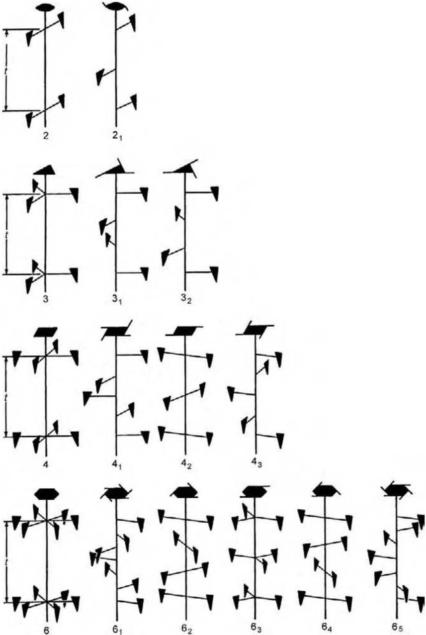
**Figure 9-19.** The eleven screw axes. The simple twofold, threefold, fourfold and sixfold axes are also shown for completeness. After Azaroff [24]; copyright (1960) McGraw-Hill, Inc.; used with permission.
