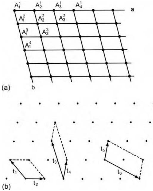
**Figure 8-26.** (a) Plane lattice defined by two non-collinear translations; (b) Illustration of primitive and unit cells on a plane lattice (after Azaroff, [38] used with permission from McGraw-Hill and L. V. Azaroff).
