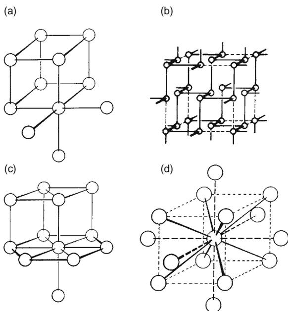
**Figure 9-26.** Examples of sphere packing after Wells [39]. Reproduced with permission. (a) Simple cubic; (b) The somewhat distorted cubic packing of arsenic; (c) Simple hexagonal; (d) Body-centered cubic.
