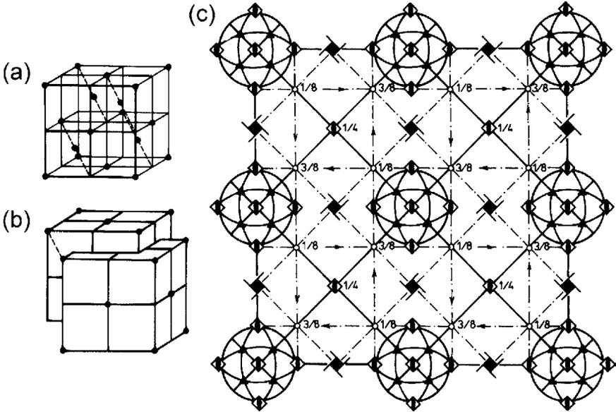
**Figure 9-23.** The diamond structure after Shubnikov and Koptsik [33]. (a) A unit cell; the edges of the cube are the  $a$ ,  $b$ , and  $c$  axes; (b) Two face-centered cubic sublattices displaced along the body diagonal of the cube; (c) Projection of some symmetry elements of the  $Fd\bar{3}m$  space group onto a horizontal plane. The vertical screw axes  $4_1$  and  $4_3$  are marked by appropriate symbols. Used with permission.
