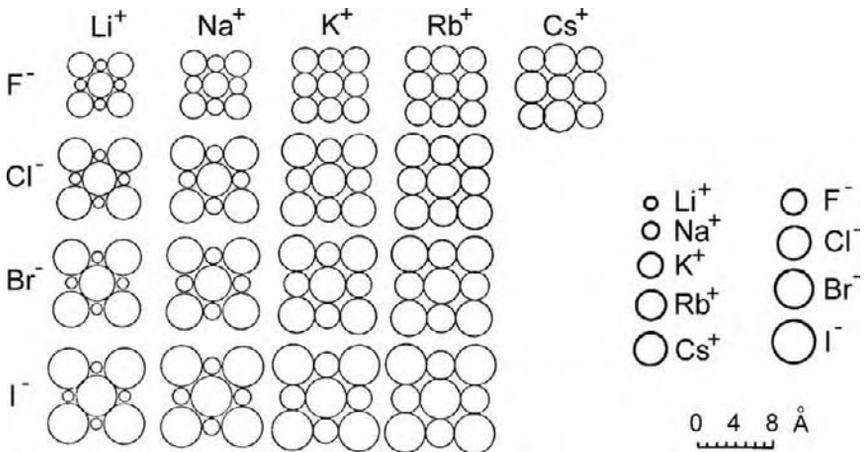
**Figure 9-41.** The arrangement of ions in cube-face layers of alkali halide crystals with the sodium chloride structure. Adaptation from Pauling [61]. Copyright (1960) Cornell University. Used by permission of the publisher, Cornell University Press.
