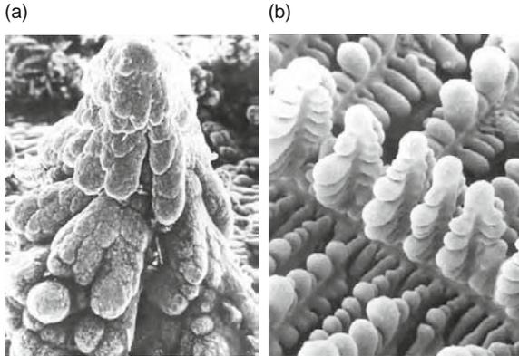
**Figure 2-9.** (a) Electrolytically deposited copper, magnification  $\times 1000$ . Courtesy of Maria Kazinets, Beer Sheva; (b) Directionally solidified iron dendrites from an iron-copper alloy after dissolving away the copper, magnification  $\times 2600$ . Courtesy of J. Morral, Storrs, Connecticut.
