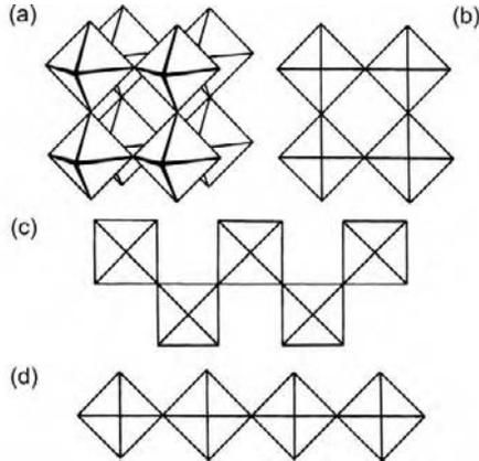
**Figure 9-36.** Connected octahedra: (a) and (b) Two representations of four octahedra sharing adjacent vertices and forming a tetramer; (c) Infinite chain of octahedra connected at adjacent vertices; (d) Infinite chain of octahedra connected at nonadjacent vertices.
