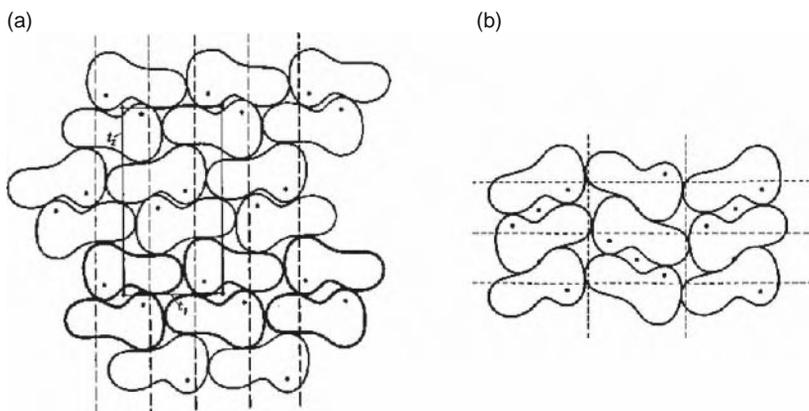
**Figure 9-50.** Two forms of packing with  $pgg$  space groups after Kitaigorodsky [91]. (a) Densest packing of molecules with arbitrary shape; (b) Another orientation of the molecules which reduces the coordination number to four.
