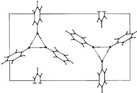
**Figure 9-55.** The molecules in the phenol crystal are connected by hydrogen bonds and are forming spirals with a threefold screw axis. This symmetry element is not part of the three-dimensional space group of the phenol crystal. After Zorky and Koptsik [103].
