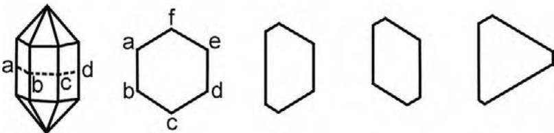
**Figure 9-5.** Sections of ideal and distorted quartz crystals.
