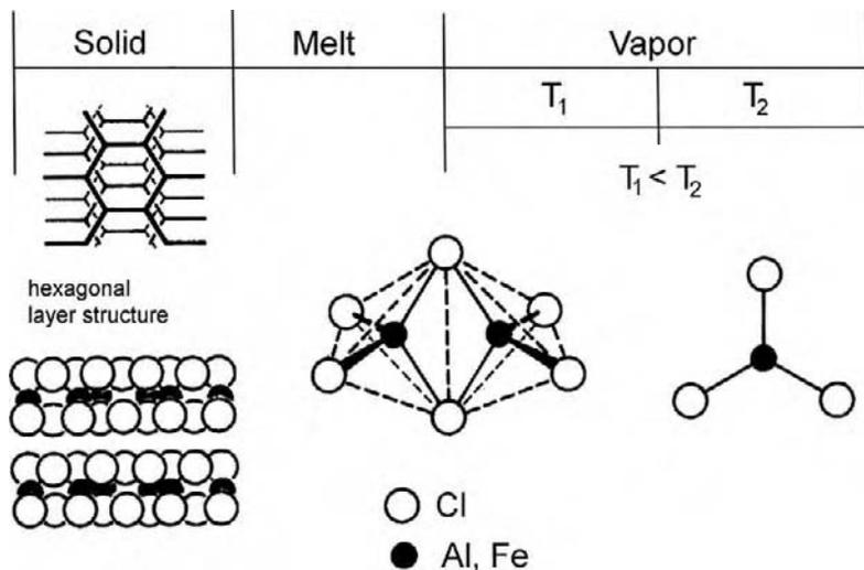
**Figure 9-58.** Structural changes upon evaporation of aluminium trichloride.
