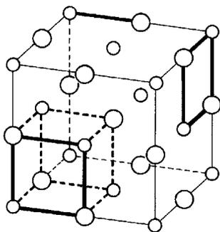
**Figure 9-56.** Part of sodium chloride crystal structure with  $\text{NaCl}$ ,  $(\text{NaCl})_2$ , and  $(\text{NaCl})_4$  units indicated. The species of  $3 \times 3 \times 3$  ions itself has a high relative abundance in cluster formation.
