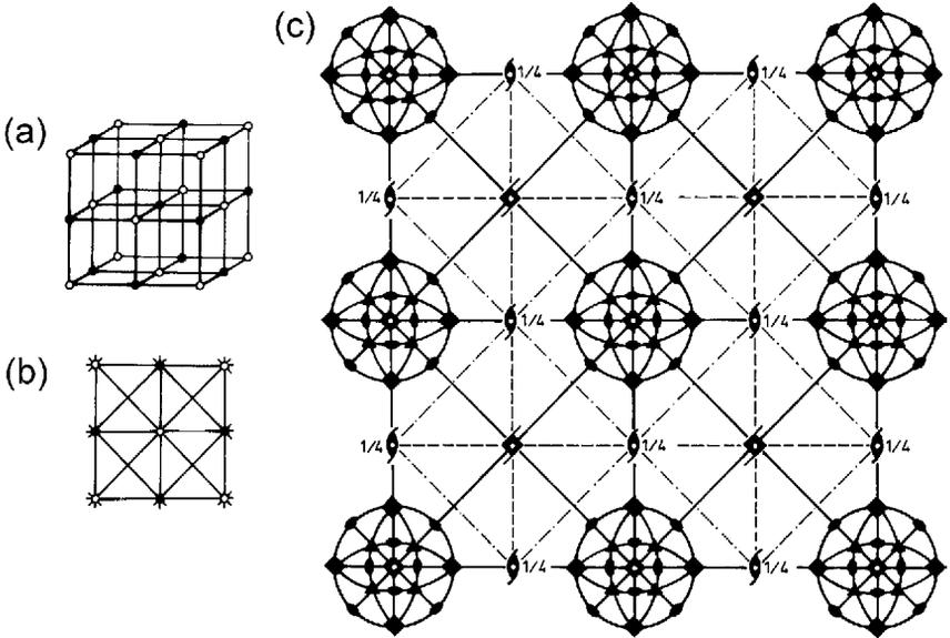
**Figure 9-22.** The crystal structure of the rock salt after Shubnikov and Koptsik [32]. (a) A unit cell; (b) Projection of the structure along the edges of the unit cell onto a horizontal plane; (c) Projection of some symmetry elements of the  $Fm\bar{3}m$  space group onto the same plane. The vertical screw axes  $2_1$  and  $4_2$  are marked by their respective symbols. Used with permission.
