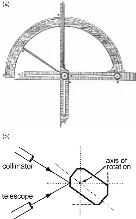
**Figure 9-6.** Goniometers; (a) Contact goniometer from Häüy [9]; (b) Scheme of reflecting goniometer.
