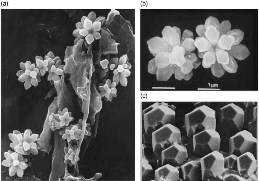
**Figure 9-64.** Quasicrystals: (a–b) Flower-like icosahedral quasicrystal in a quenched Al/Mn sample (from Csanády et al.) [152]; (c) Pentagonal dodecahedron in quasicrystalline Al/Cu/Ru obtained by slow cooling from melt (courtesy of H.-U. Nissen, Zurich) [153].
