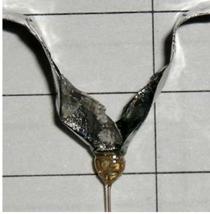
Fig. 2.8. Illustration of unsatisfactory mechanical properties of thin Pt plate used for manufacturing of the crucibles for resistively heated \mu -PD. The crucible of original shape shown in Fig. 2.3 was deformed when pulling of the crystal
