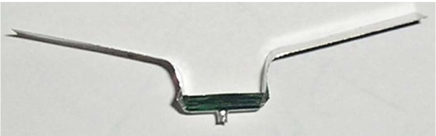
Fig. 2.3. View of \mu -PD resistive crucible manufactured at laboratory conditions. The reservoir length is 12 mm
