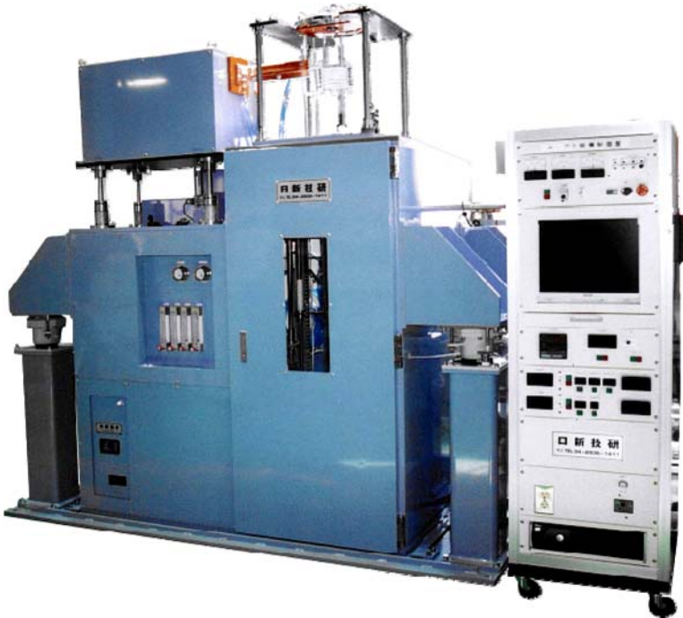
Fig. 3.17. \mu -PD system designed for the multi-crystal growth
