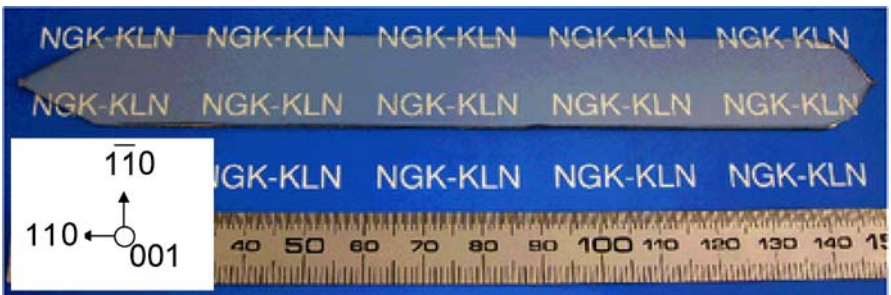
Fig. 14.4. \mu -PD KLN plate crystal (120 × 15 × 1 mm); scale in mm
