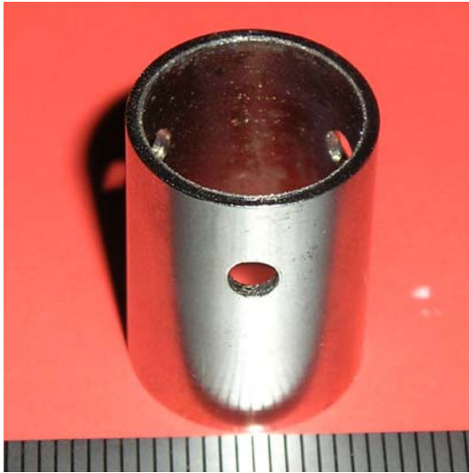
Fig. 2.15. Multi-window Ir after-heater used to improve symmetry of temperature distribution just below the crucible
