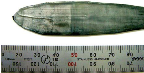
Fig. 16.8. Sapphire plate crystal grown by the \mu -PD method using molybdenum crucible
