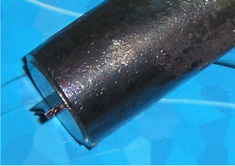
Fig. 2.13. View of bottom of Mo crucible with plate type die. The lower extremity of the die has concave shape
