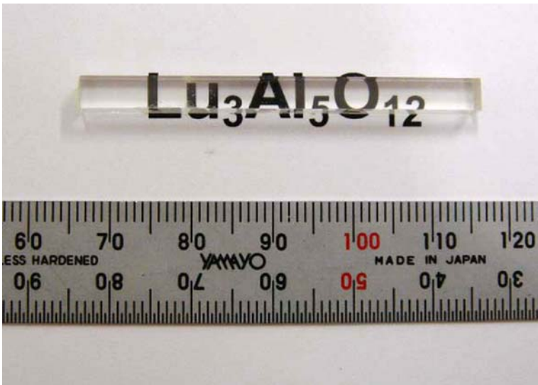
Fig. 9.16. LuAG single crystal with square rod shape grown by the \mu -PD method
