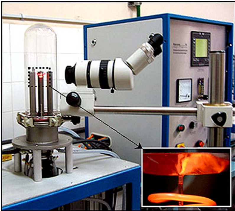
Fig. 20.2. View of adapted commercial \mu -PD system during LiF fiber pulling with Pt crucible in detail [6, 29]
