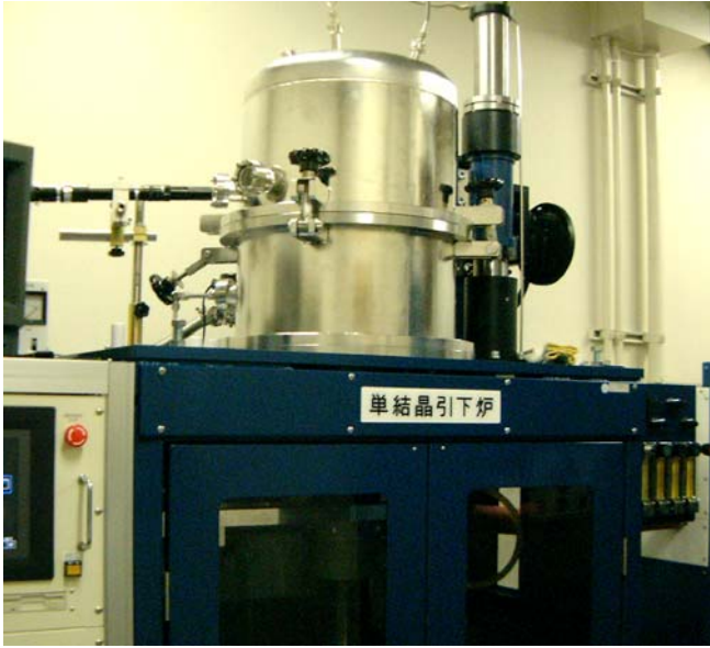
Fig. 21.2. View of \mu -PD apparatus with growth chamber designed for growth systems with aggressive \text{CF}_4 environment
