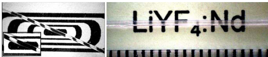
Fig. 20.4. YLF fiber grown from a melt with 5 mol% of LiF excess, with constant rate of 0.75 mm/min, under mixed flow of Ar plus CF 4 ( left ), and Nd-doped YLF fiber growth under similar conditions ( right ) [5, 6, 29]
