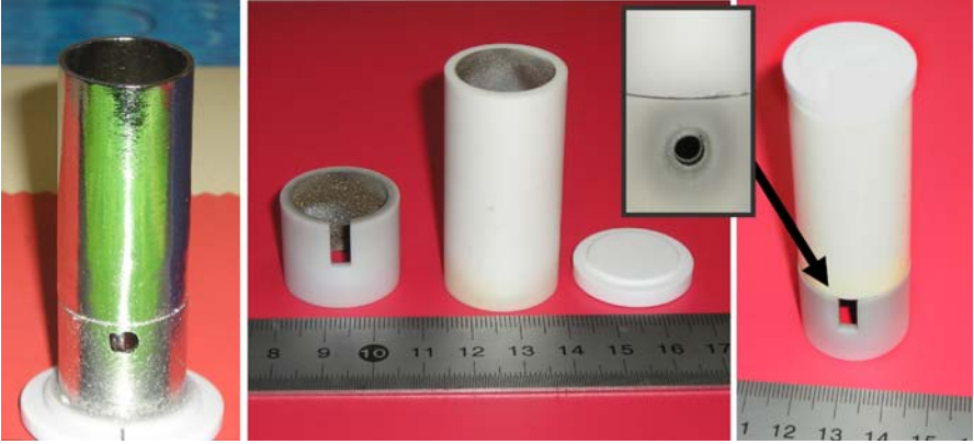
Fig. 2.6. View of the hot zone arrangement made from Ir crucible and the after-heater ( left ), typical components of the thermal insulation made of high purity \text{Al}_2\text{O}_3 ceramic ( middle ), and as assembled construction ( right ) used in inductively heated \mu -PD (Scales in mm)
