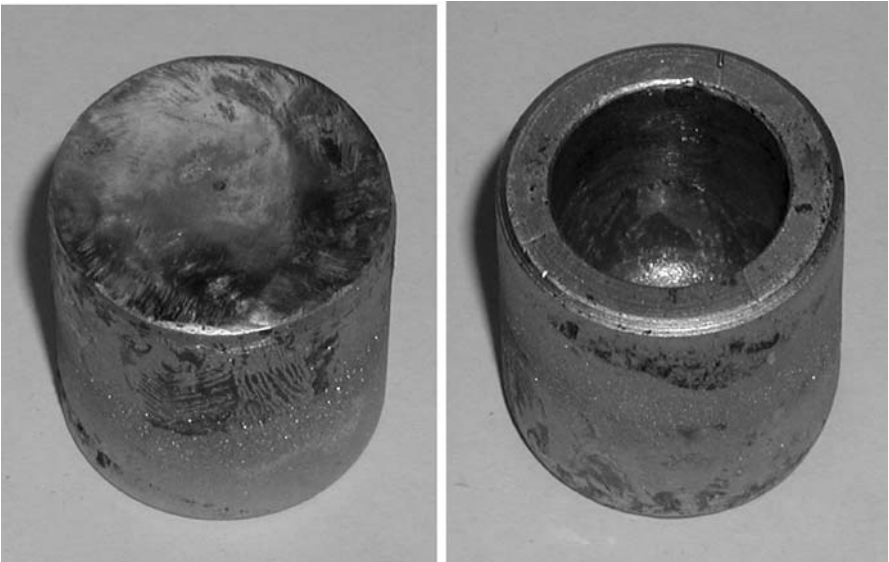
Fig. 1.13. Porous Ir die ( \varnothing 27 mm) used in pulling-up EFG process. Left view represents actual position of the die in the growth (Fig. 1.12, right ). The die was used for the growth of rare-earth vanadate crystals with details available in [36] (Courtesy of V.V. Kochurikhin, 2005)
