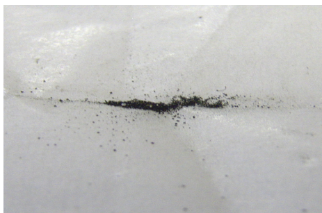
Fig. 8. A photograph of the deposits recovered by electrochemical reduction of uranyl species in BMINfO.
