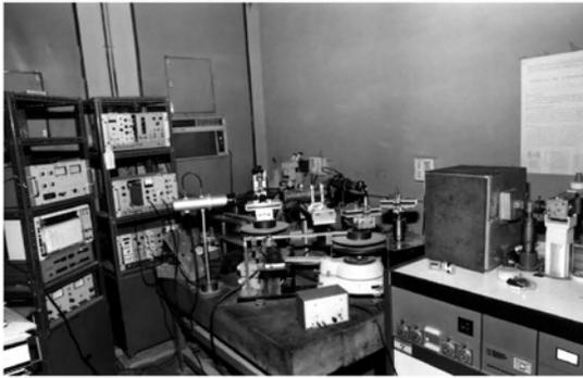
**Fig. 12.7.** A photograph of the five crystal X-ray diffractometer, designed, developed, and fabricated at NPL
