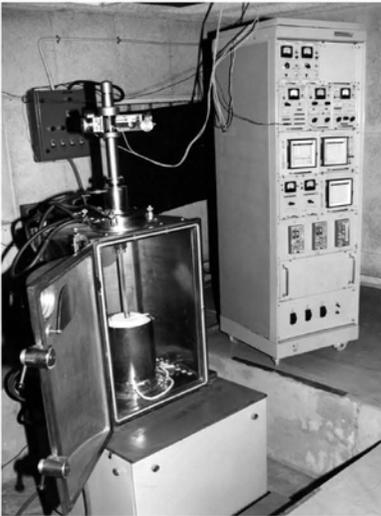
**Fig. 12.3.** A photograph of the crystal growth system employed for growth of crystals by the low thermal gradient Cz method
