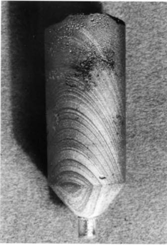
**Fig. 15.5.** ZnSe crystal grown by high pressure Bridgman method (from Reference 41)
