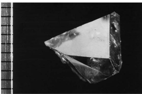
**Fig. 15.12.** ZnSe crystal grown by chemical vapor transport with iodine as chemical agent (from Reference 92) (scale in mm)
