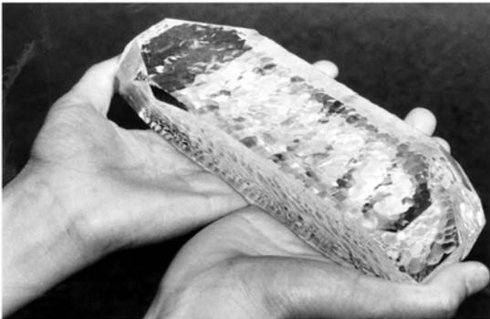
Fig. 17.7. Quartz crystal hydrothermally grown
