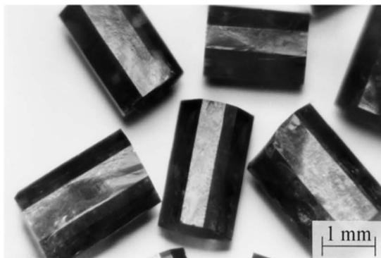
**Fig. 17.9.** Emerald crystals grown from  $\text{Li}_2\text{O-MoO}_3$  flux
