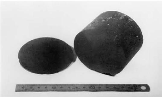
**Fig. 15.1.** 80-mm diameter ZnTe single crystal (from Reference 9)
