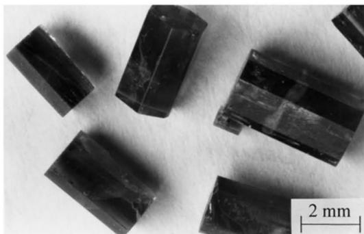
**Fig. 17.12.** Large emerald crystals grown from  $K_2O$ - $MoO_3$  flux
