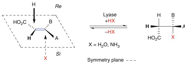
**Scheme 2.210** Lyase-catalyzed addition of water and ammonia onto activated  $\text{C}=\text{C}$  bonds
