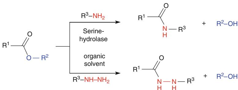
Scheme 3.21 Ammonolysis, aminolysis, and hydrazinolysis of esters
