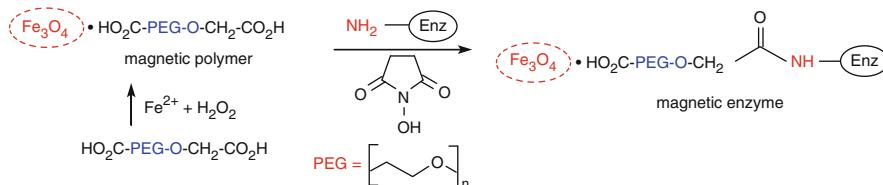
**Scheme 3.41** Modification of enzymes by magnetite-polyethylene glycol
