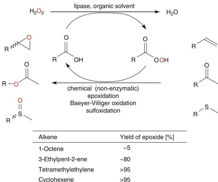
**Scheme 3.29** Lipase-catalyzed peracid formation and catalytic epoxidation
