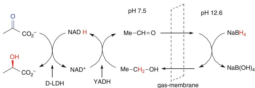
**Scheme 3.39** Cofactor recycling using a gas-membrane reactor
