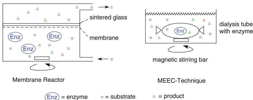
**Fig. 3.7** Principle of a membrane reactor and the membrane-enclosed enzyme catalysis (MEEC)-technique
