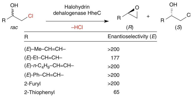
Scheme 2.237 Kinetic resolution of halohydrins using halohydrin dehalogenase
