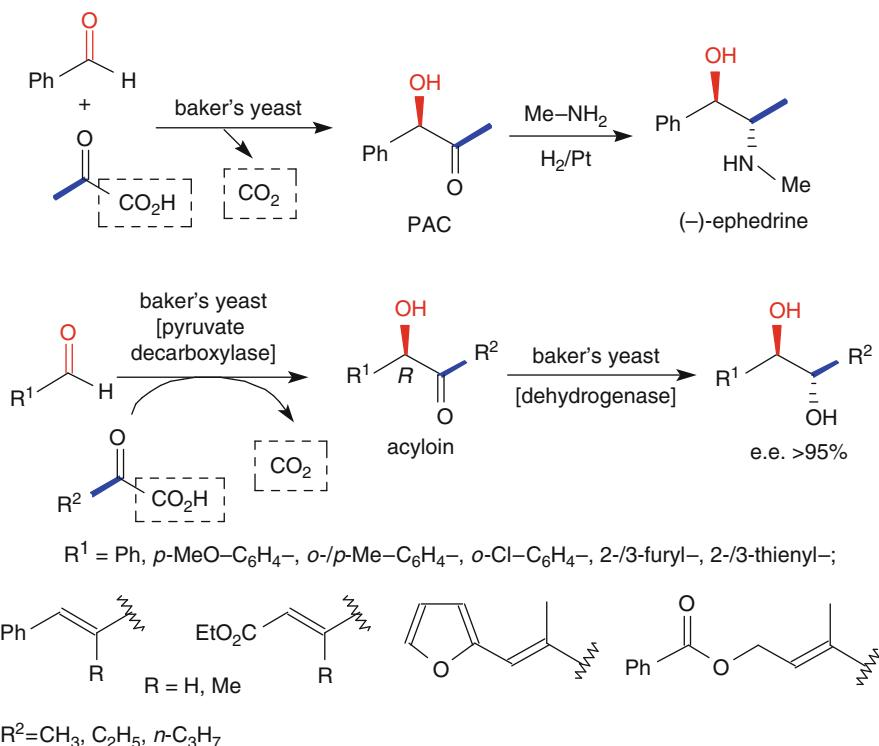
**Scheme 2.199** Synthesis of (−)-ephedrine via baker's yeast catalyzed acyloin reaction and acyloin formation catalyzed by pyruvate decarboxylase
