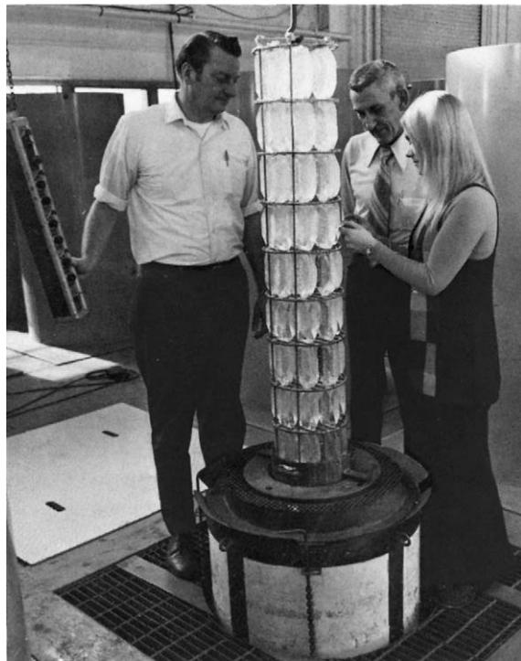
Fig. 2. Harvesting an early quartz growth run, AT&T Merrimac Valley Factory, Massachusetts.
