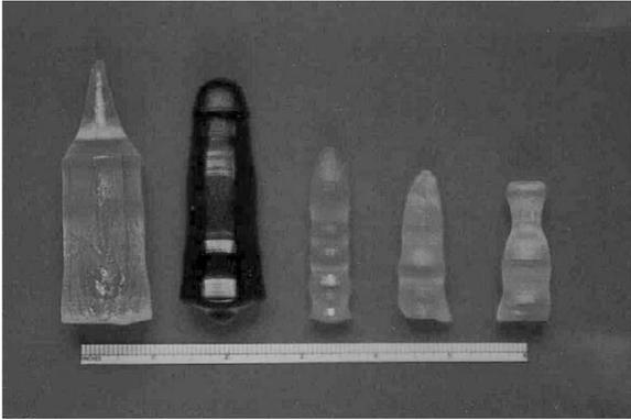
Fig. 12. Early garnet crystals grown using RF power pickup and diameter control based on visual observations.
