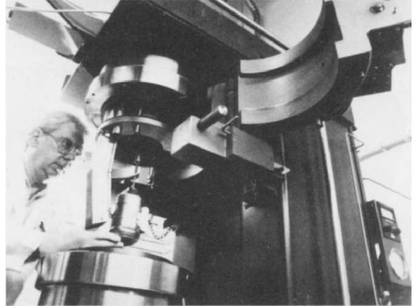
Fig. 3. Removal of GaAs boule from furnace after growth.
