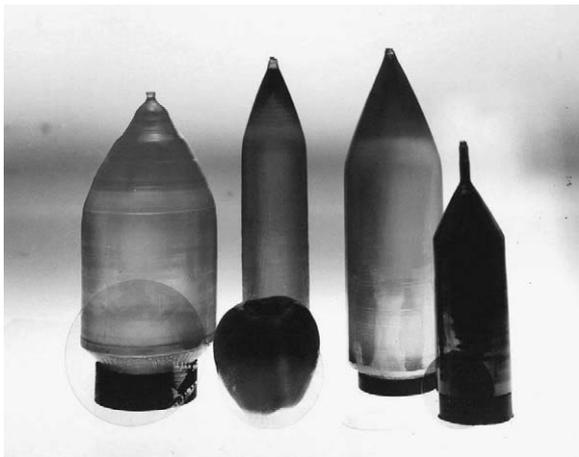
Fig. 14. Current examples of large diameter perovskite crystals that were grown using the crystal weighing technique with digital control.
