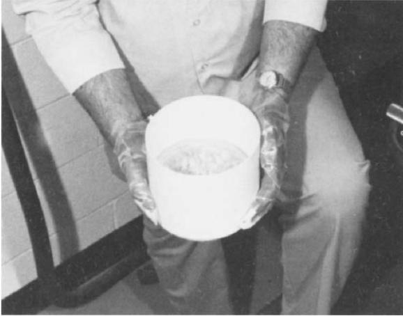
Fig. 2. Pyrolytic boron nitride CPBN crucible with premelted charge.
