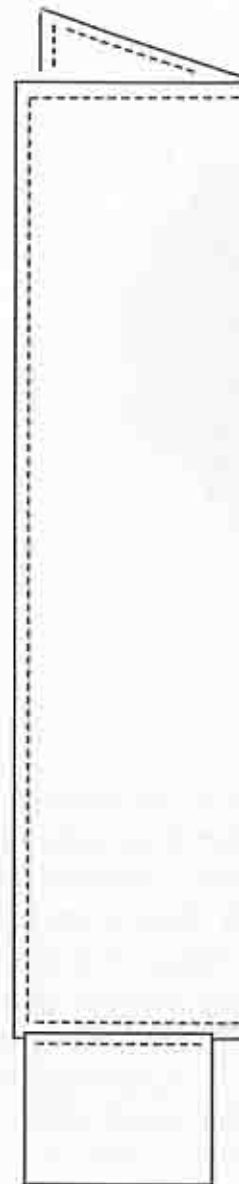
Figure 3-3. Fold the material lengthwise and sew the bottom and open edge closed. Sew or glue the netting and garnish.
